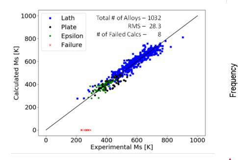
Comparison of calculated Ms against experimental Ms temperatures. Alloy compositions and Ms temperatures compiled from literature by Hanumantharaju.
