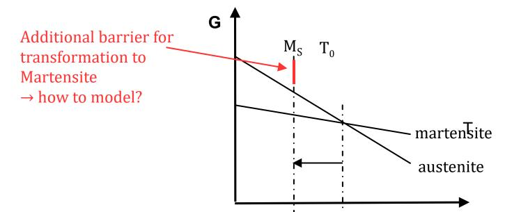
Semi-empirical model for describing the additional barrier (Stormvinter et al. Met. Mater Trans. 43A (2012)):
