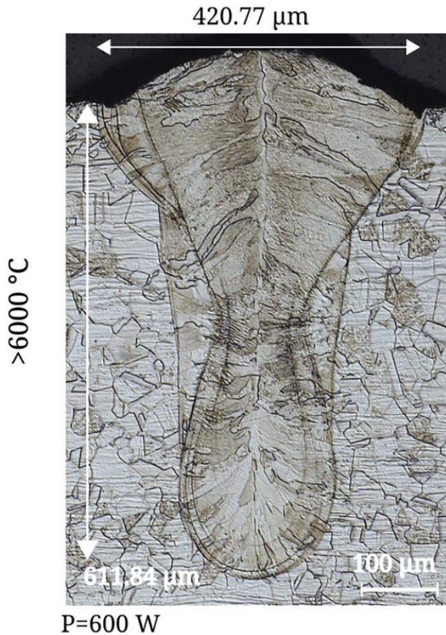
Figure 153: Cross-section showing the experimental melt track for the same processing conditions shown in Figure 152. From [2024Hol-Fig9].
