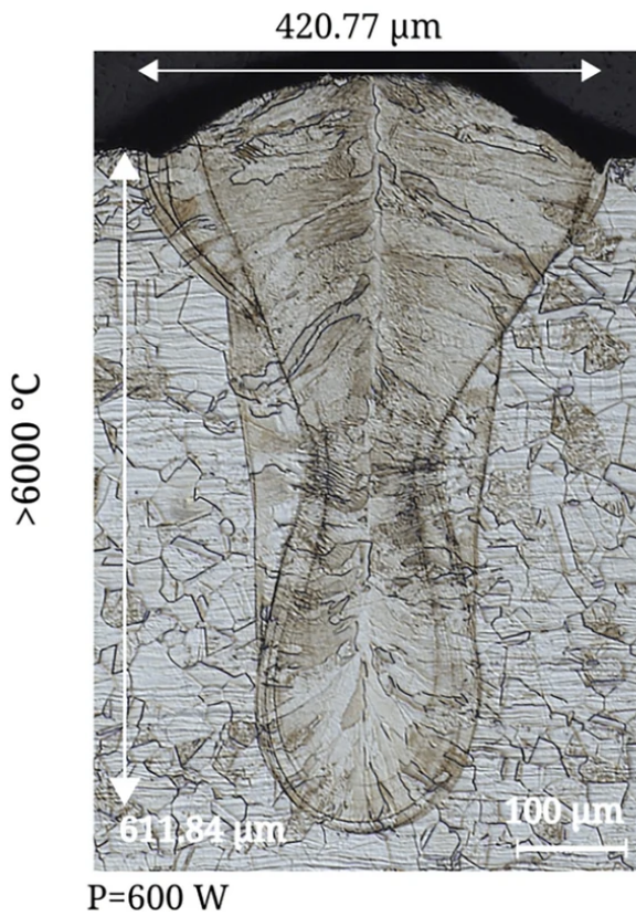
Figure 135: Cross-section showing the experimental melt track for the same processing conditions shown in Figure 134. From [2024Hol-Fig9].
