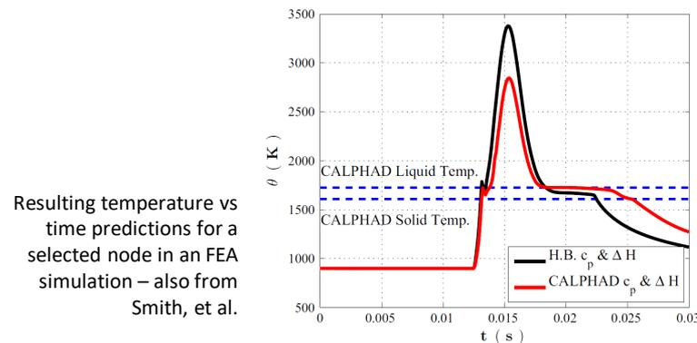
Resulting temperature vs time predictions for a selected node in an FEA simulation – also from Smith, et al.
