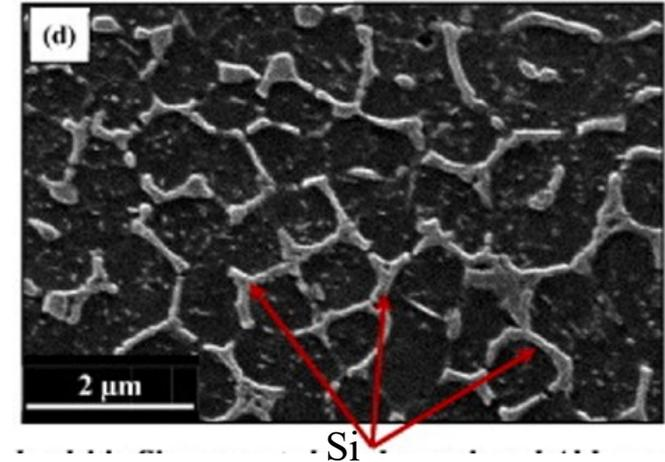
Microstructure of SLM Al10SiMg
