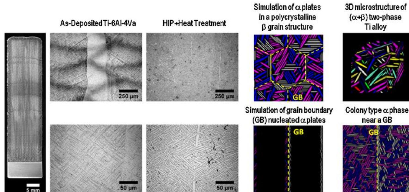
Example of phase field model compared with build microstructure – from *R. Martukanitz et al. / Additive Manufacturing 1–4 (2014) 52–63*
