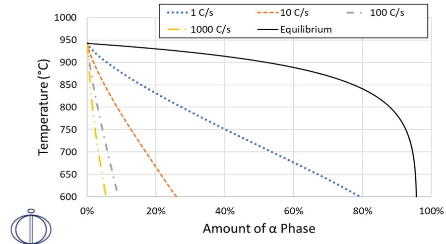
Calculated phase fraction of alpha for a B homogenized Ti-6-4Al alloy during continuous cooling through diffusion controlled simulations.
