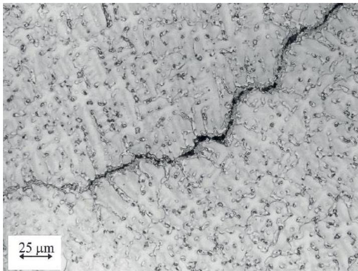
Left: Solidification crack along solidification grain boundary in Ni-base alloy weld
