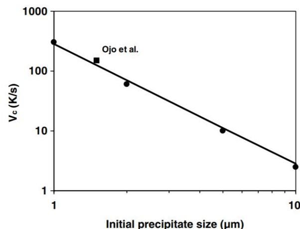
Fig. 5. Variation of the critical heating rate for  $\gamma'$  liquation,  $V_c$ , with initial precipitate size.
