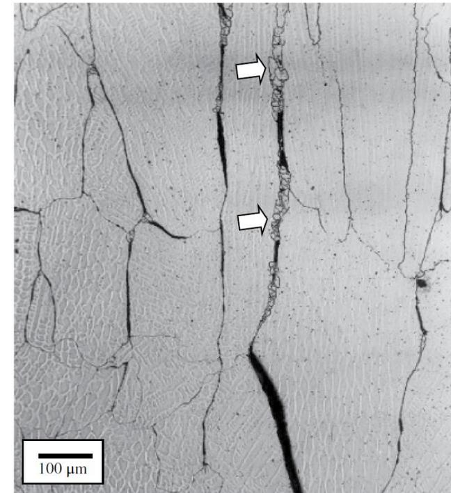
Right: Ductility dip cracks along migrated grain boundaries in Ni-base alloy multi-pass weld
