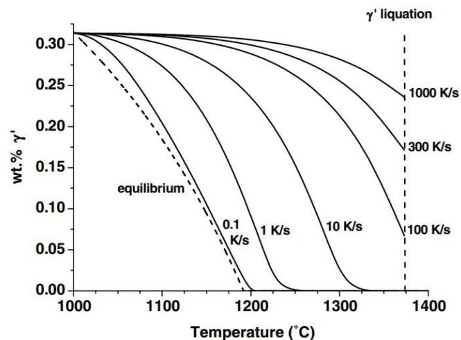
Fig. 3. Evolution with temperature of the relative amount of  $\gamma'$  during heating at different rates.
