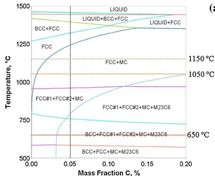
Above: Isoleth section showing that even with variation in carbon, a large FCC+MC carbide region can be found to perform homogenization treatment
