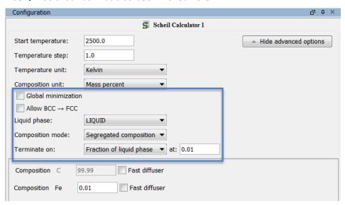
For the Scheil Calculator, the method for calculating the segregation is the same as before but with an improvement to what and how the simulation results are stored.
