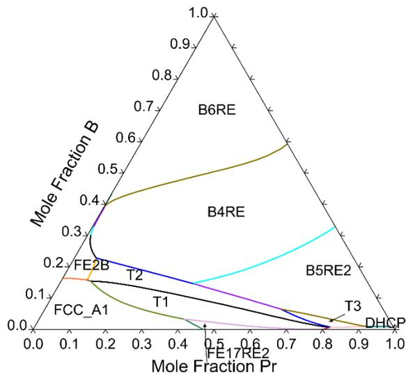
Figure 12: Calculated Fe-Pr-B liquidus projection.
