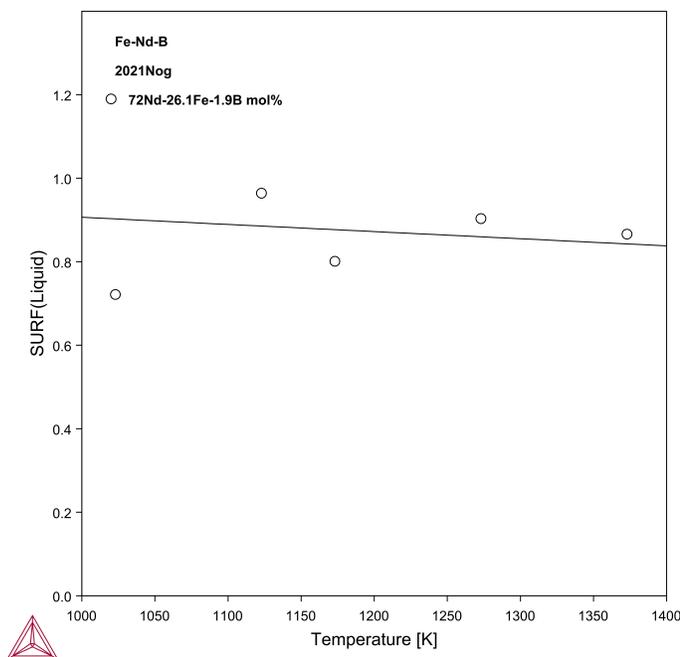
Figure 13: Calculated surface tension of Nd-Fe-B ternary alloy compared with experimental data from [2021Nog].
