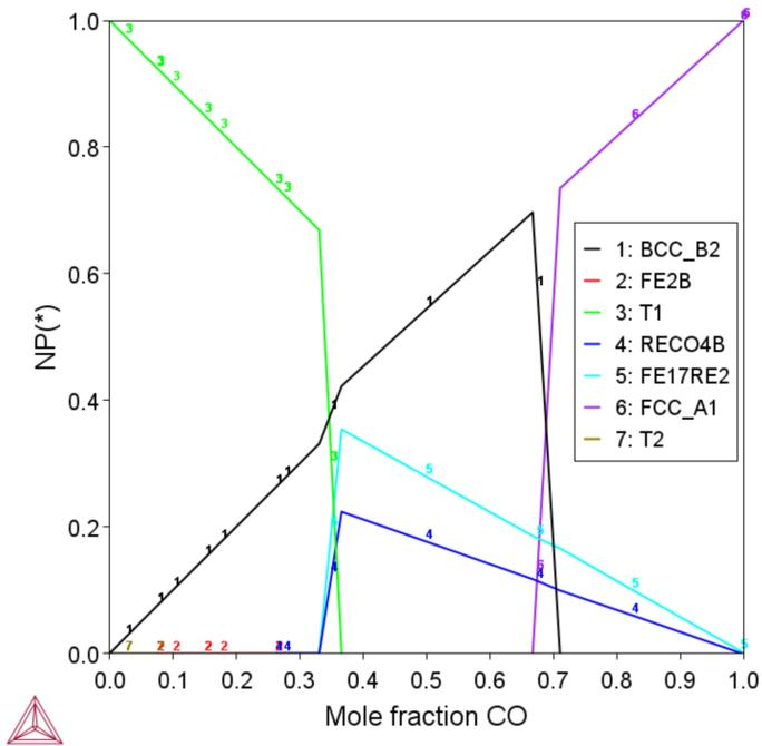
Figure 1: Calculated  $Ce_2Fe_{14}B$ -Co step diagram at 900 °C.
