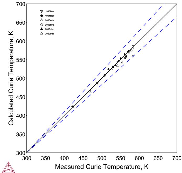
Figure 3: Comparison of calculated vs experimental Curie temperatures.
