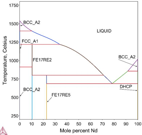
Figure 6: Calculated Fe-Nd phase diagram.
