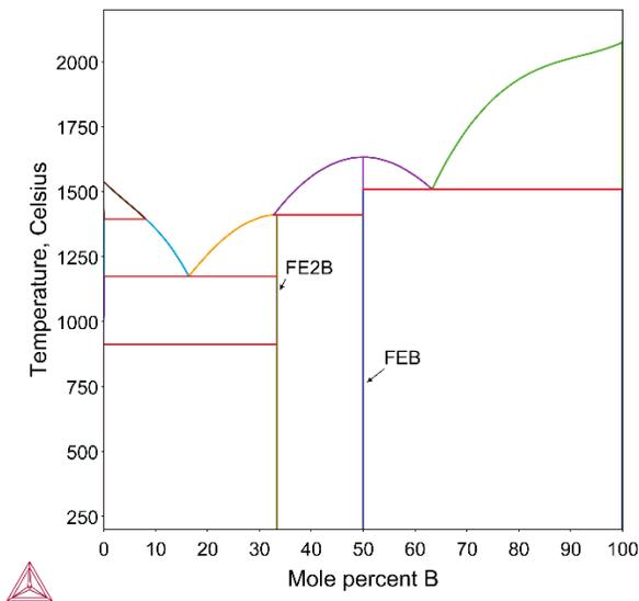
Figure 5: Calculated Fe-B phase diagram.
