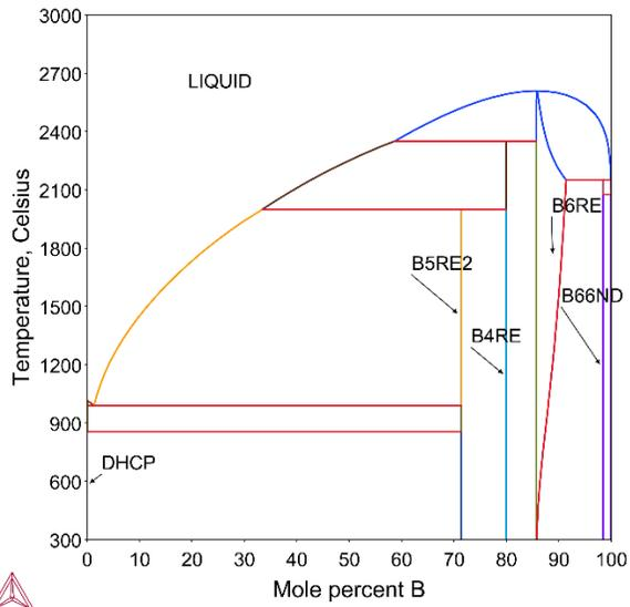
Figure 7: Calculated Nd-B phase diagram.
