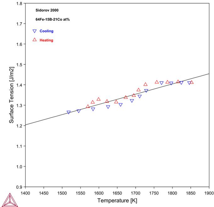
Figure 14: Calculated surface tension of B-Co-Fe ternary alloy compared with experimental data from [2000Sid].
