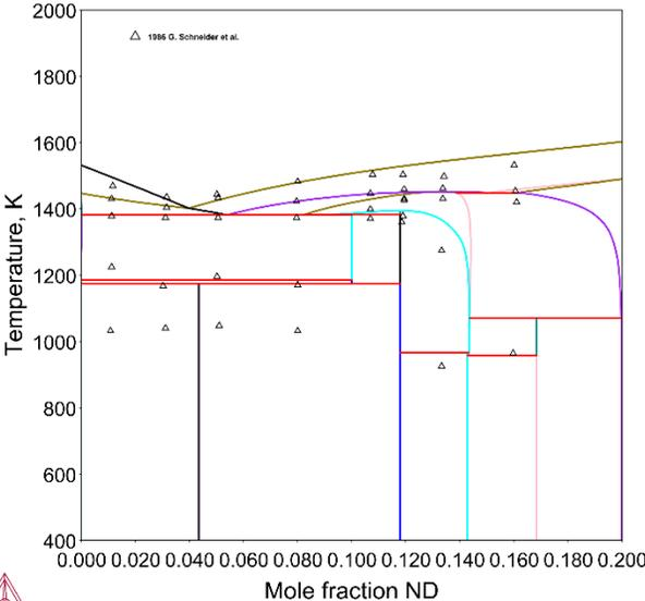
Figure 10: Calculated vertical section of Fe-Nd-B at 80 at. % Fe with experimental data from [1986Sch].
