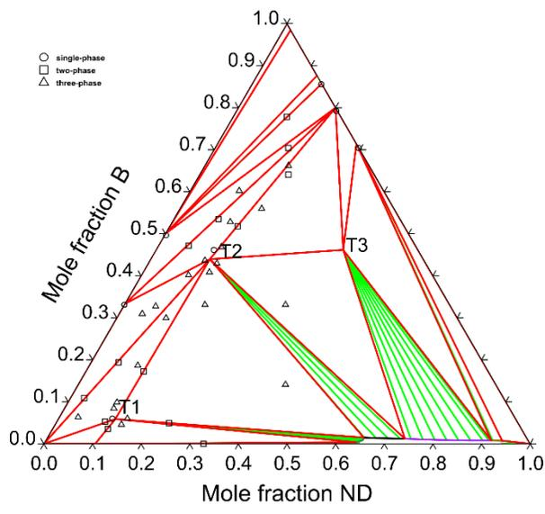
Figure 9: Calculated Fe-Nd-B isothermal section at 1173 K with experimental data from [1985Bus] and [1986Bus].
