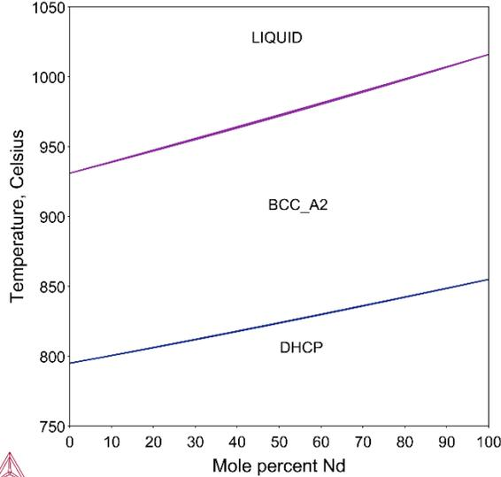
Figure 8: Calculated Nd-Pr phase diagram.
