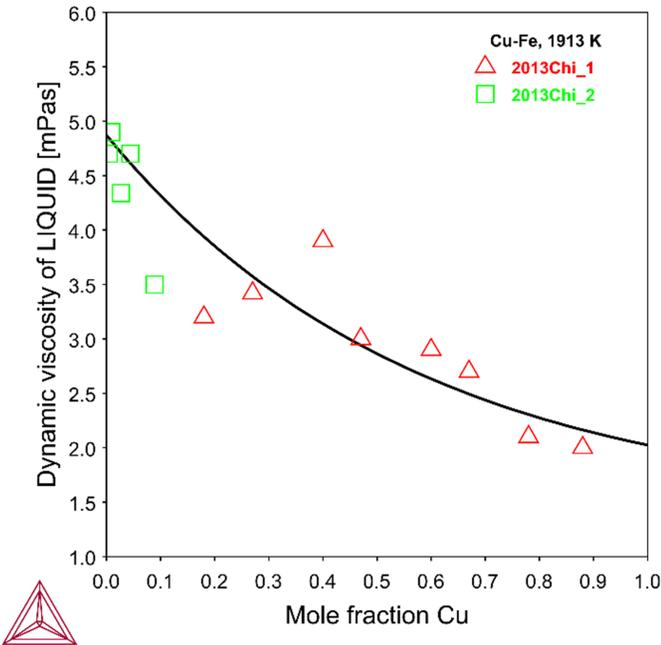
Figure 17: Calculated dynamic viscosity of Cu-Fe at 1913 K along with experimental data from [2013a/bChi].
