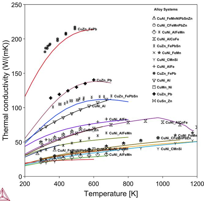
Figure 26: Thermal conductivity versus temperature for various Cu-based alloys, e.g. CuNi\_AlFeMn indicates the Cu-alloy with Ni as the major alloying element and Al, Fe, and Mn the minor alloying elements. Experimental data from [1991Lan]. Curves: Frozen-in calculations by the latest version of the database.
