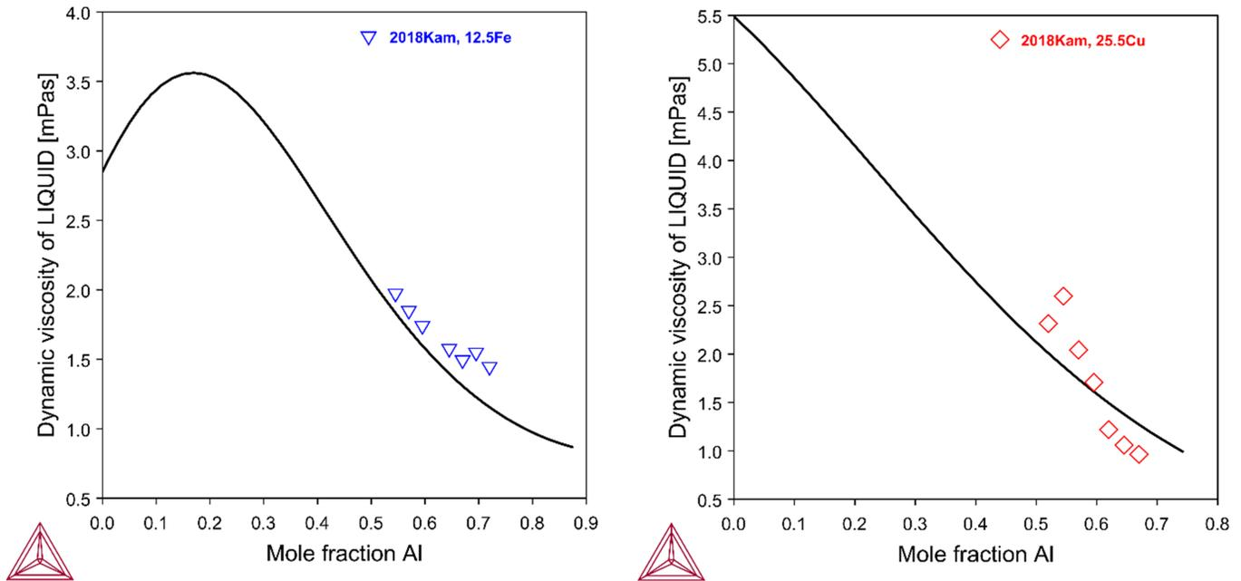
Figure 18: Kinematic viscosity of Al-Cu-Fe alloys at 12.5 at% Fe (left) and 25.5 at% Cu (right) along with experimental data from [2018Kam].
