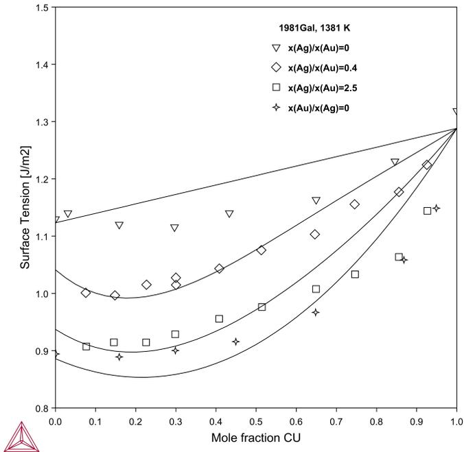
Figure 15: Calculated surface tension of Ag-Cu, Au-Cu and Ag-Au-Cu alloys at 1381 K along with experimental data from [1981Gal].
