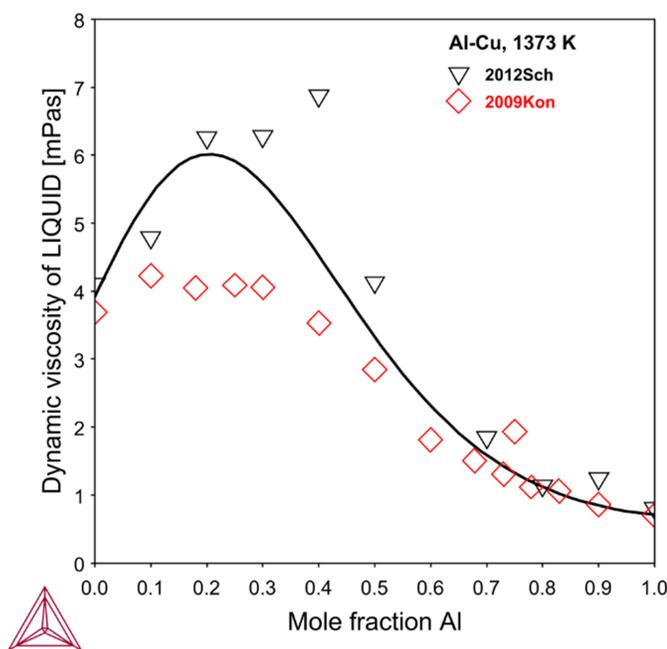
Figure 16: Calculated dynamic viscosity of Al-Cu at 1373 K along with experimental data from [2009Kon; 2012Sch].
