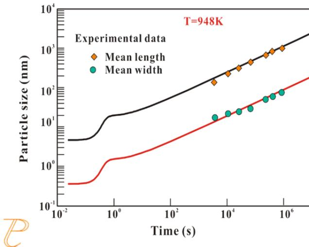
Figure 22: Simulated average length (red line) and width (black line) of rod-shaped precipitates with aging time for Cu-1.86wt.%Ni-0.45wt.%Si alloy at 948K compared with reported experimental data [2011Wat].
