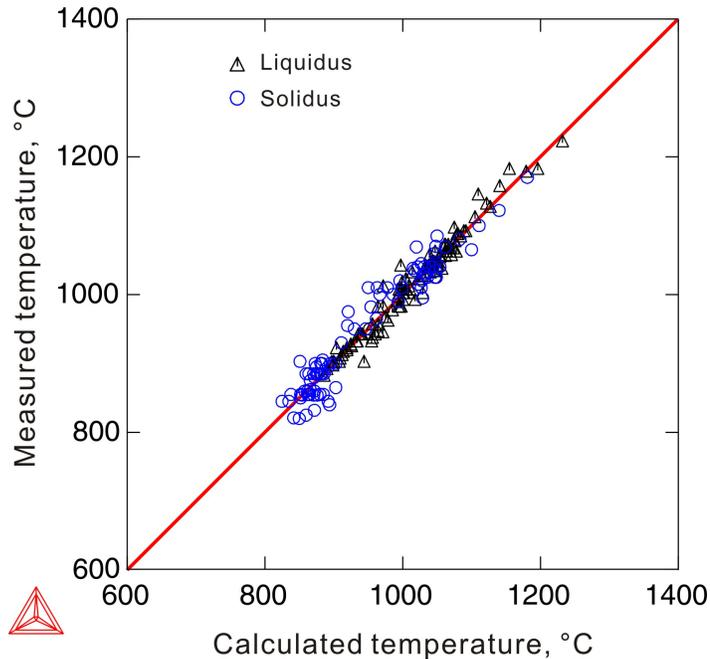
Figure 19: Comparison of calculated and experimental [2001Dav] liquidus and solidus temperatures for various industry copper alloys.
