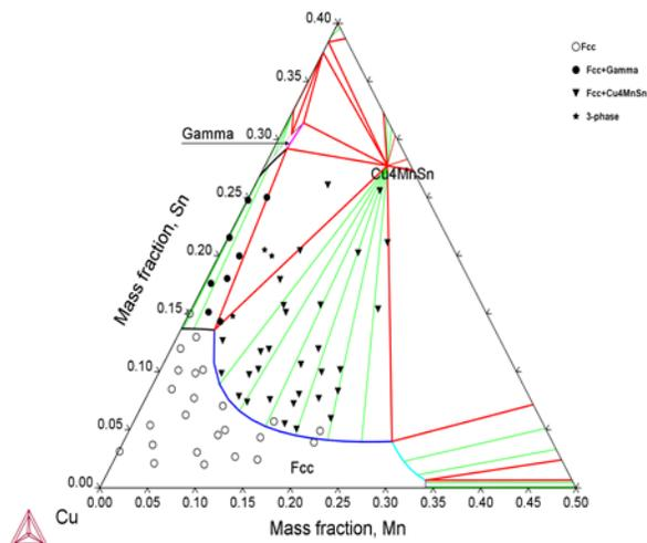
Figure 5: Calculated isothermal section of Cu-Mn-Sn at 550°C along with experimental data [1953Bla; 1953Fun; 1987Leo].
