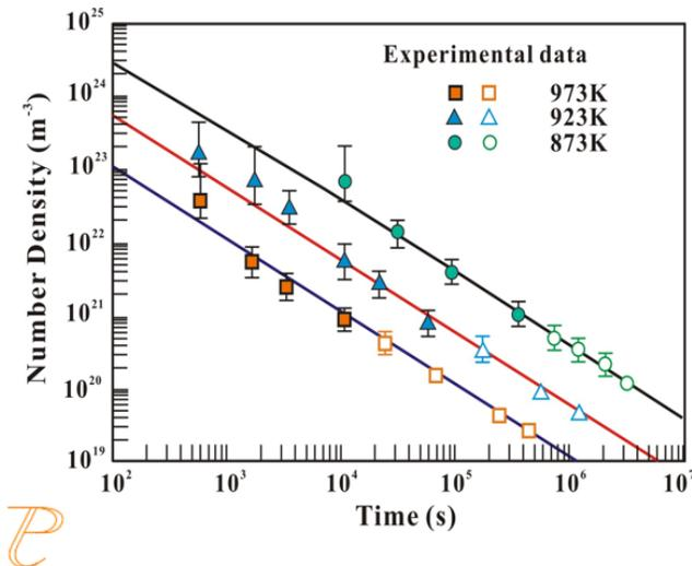
Figure 24: Simulated and experimental number density of fcc Co-Fe precipitate in Cu-0.68 at.%Co-1.52 at.%Fe alloy annealed at 973, 923, and 873 K. The solid symbols are experimental data [2009Wat] for spherical particles; and the open symbols are for cuboid particles.
