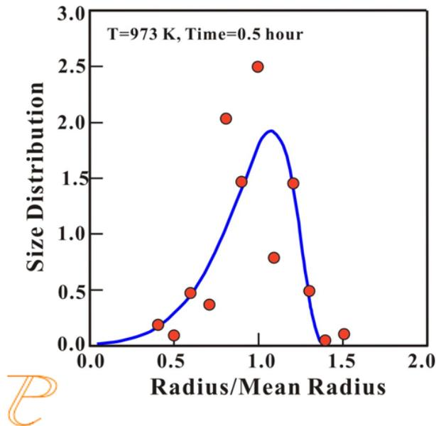
Figure 23: Comparison of the simulated particle size distribution of fcc Co-Fe precipitates in Cu-0.68 at.%Co-1.52 at.%Fe alloy annealed at 973 K for 0.5 h with the experimental data [2011Wat].
