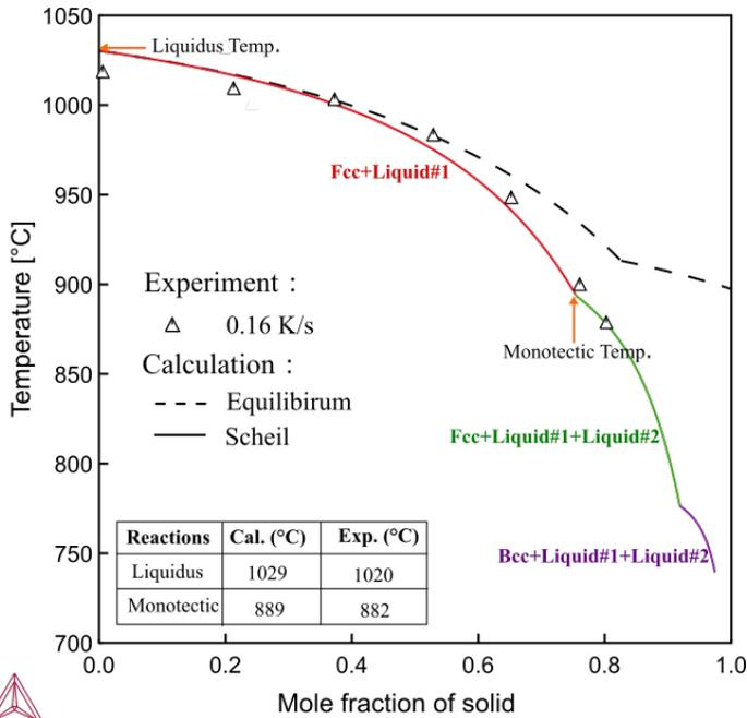
Figure 20: Equilibrium solidification and Scheil solidification simulations of Cu-5.2 wt.%Sn-4.7wt.%Pb alloy, compared with experimental result [2009Kor]. The calculated Scheil solidification path, including the solidified phases and the phase transformation temperatures, agrees well with the experimental data.
