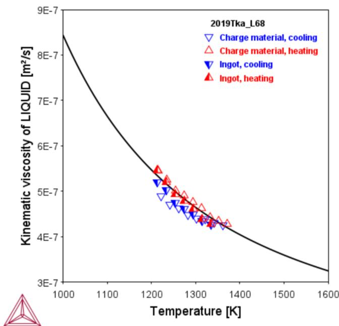
Figure 25: Calculated kinematic viscosities of the melts of L68 brass along with experimental data from [2019Tka].
