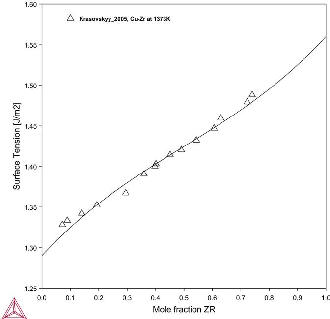
Figure 14: Surface tension of Cu-Zr at 1373 K. Experimental data are taken from [2005Kra].
