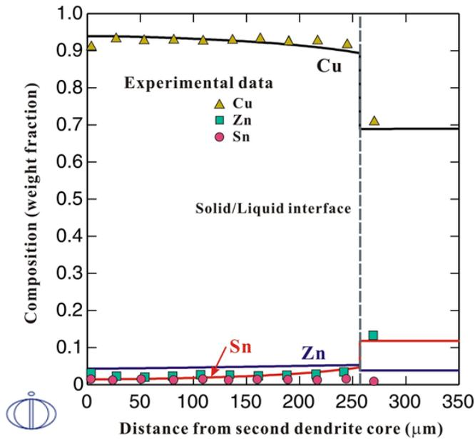
Figure 21: Calculated composition profile through half dendrite cross section in Cu-4.9wt.%Pb-5.2wt.%Sn-4.5wt.%Zn alloy during the solidification process along with experimental data [2009Kor]. The cooling rate is 0.16 °C/s.
