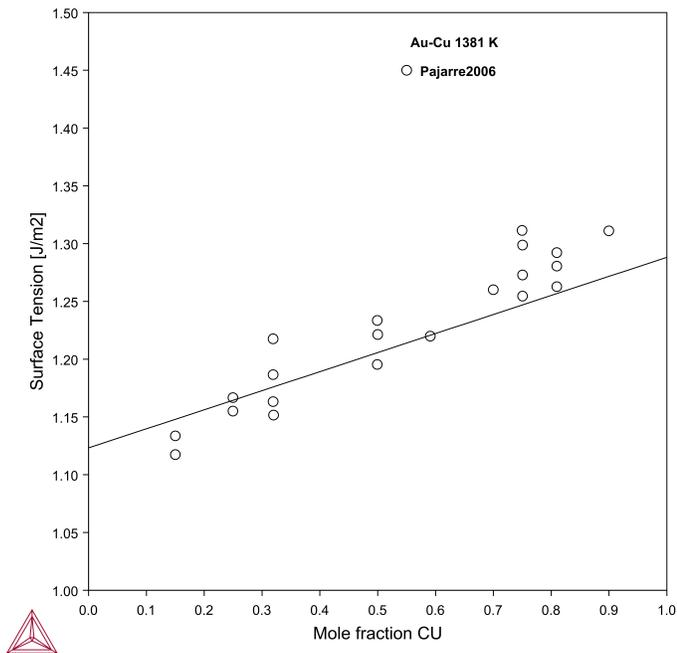
Figure 13: Surface tension of Au-Cu at 1381 K. Experimental data are taken from [2006Paj].
