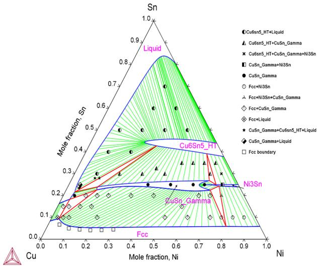
Figure 6: Calculated isothermal section of Cu-Ni-Sn at 800 °C along with experimental data [2003Wan].
