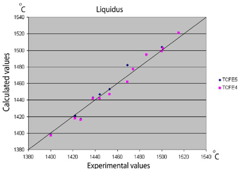
*Fig. 3: Experimental liquidus temperatures for various steels (stainless steels, carbon and low alloy steels, high-speed steels and Chromium steels) compared with calculations performed using the TCFE5 and TCFE4 databases.*
