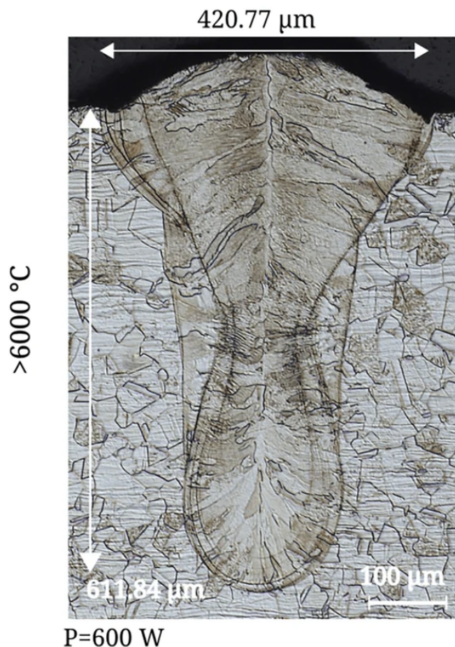
Figure 139: Cross-section showing the experimental melt track for the same processing conditions shown in Figure 138. From [2024Hol-Fig9].
