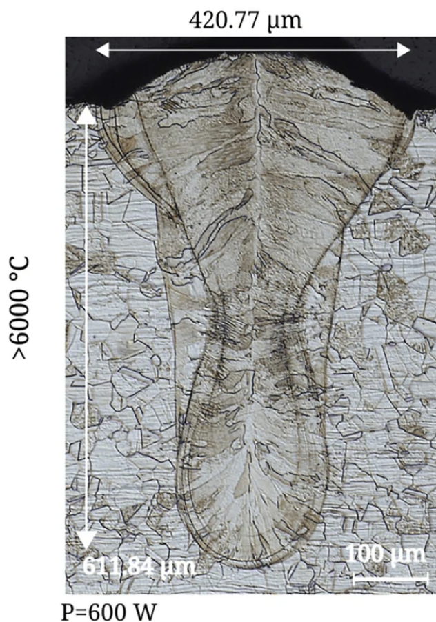
Figure 82: Cross-section showing the experimental melt track for the same processing conditions shown in Figure 81. From [2024Hol-Fig9].
