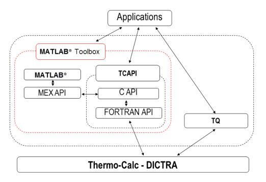
The thermodynamic properties and phase equilibrium data that can be obtained by using the TQ-Interface include Gibbs energy, enthalpy, entropy, heat capacity, first and second derivatives of Gibbs energy with respect to composition, chemical potential, phase amount, phase composition, partition coefficients, liquidus or solidus points, invariant temperature, heat of reaction, adiabatic combustion temperature, and volume, etc.
