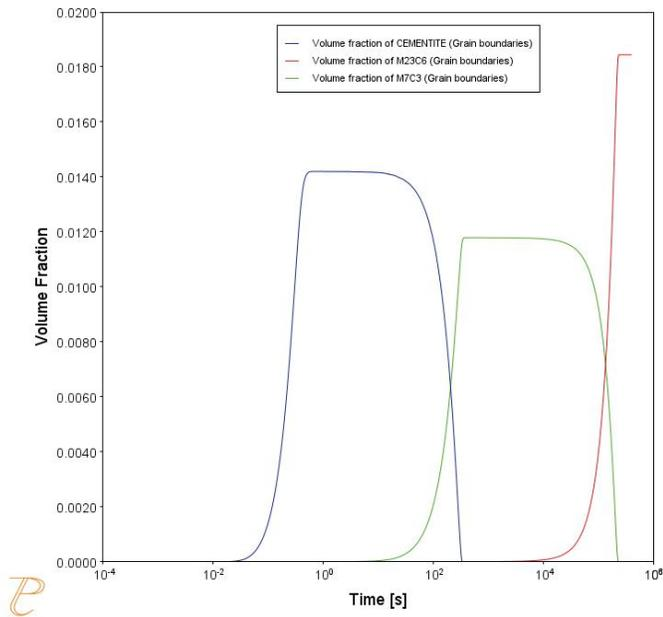
Figure 103: Volume fraction with no initial particle size distribution (PSD).
