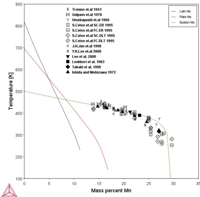
Figure 39: A diagram showing all the  $M_s$  temperatures of different types of martensite morphologies (lath, plate and epsilon (HCP)) compared with experimental epsilon  $M_s$  values.
