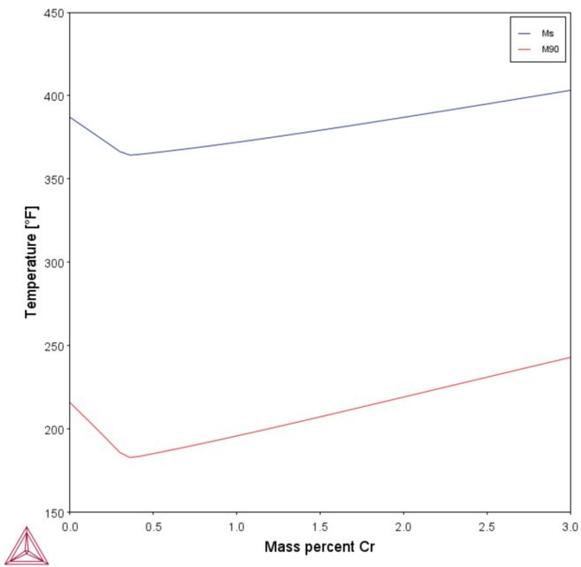
Figure 38: Comparing Martensite start (Ms) to Martensite finish (Mf).
