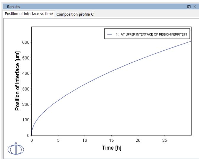
Figure 60: Position of interface vs time.
