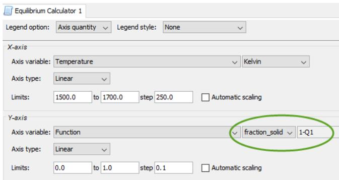
The screenshot shows the configuration window for the Equilibrium Calculator. The X-axis is set to Temperature (Kelvin) with a linear scale from 1500.0 to 1700.0 and a step of 250.0. The Y-axis is set to Function with a linear scale from 0.0 to 1.0 and a step of 0.1. The function selected for the Y-axis is *fraction\_solid*, which is circled in green. The legend option is set to Axis quantity and the legend style is set to None.
