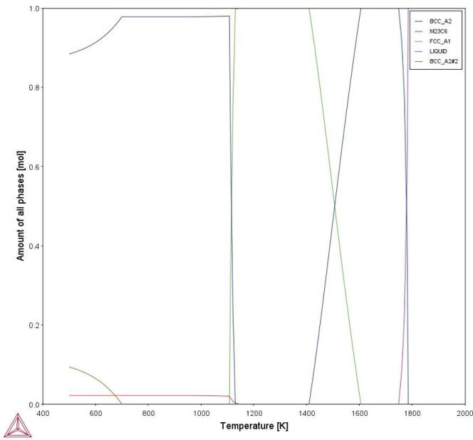
Figure 81: The Equilibrium Calculator is used to show how the phases change with temperature.
