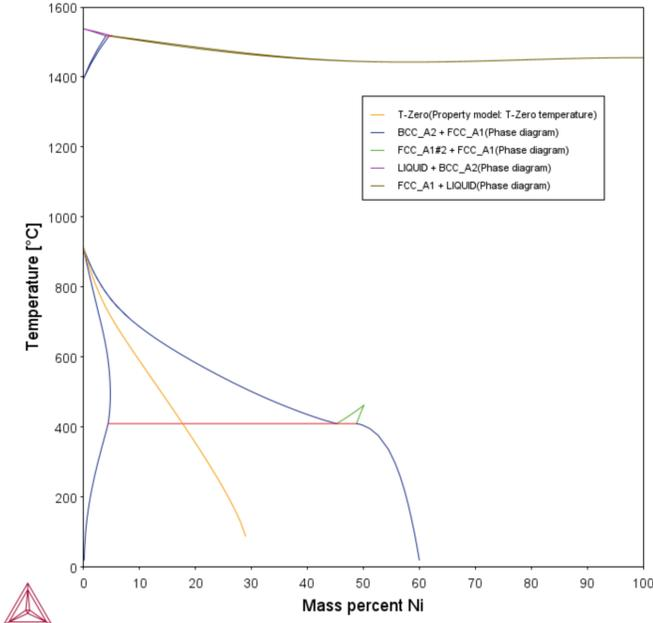
Figure 33: In this plot for the Fe-Ni system, the  $T_0$  line for the FCC\_A1 and BCC\_A2 phases is located in the middle of the two-phase region. No solution for the  $T_0$  temperature exists above about 30 mass% Ni.
