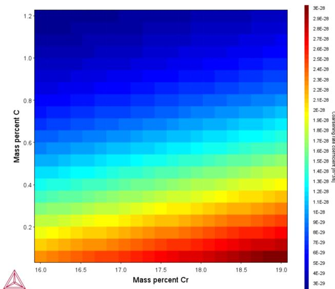
Figure 20: Coarsening rate coefficient (heat map plot).
