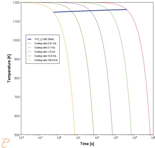
Figure 91: In this plot, the blue horizontal line shows the time it takes for  $\gamma'$  to transform at each of the cooling rates according to the stop criteria, which is set as  $1e-4$  volume fraction. The cooling rates are represented by the multicoloured curved lines.
