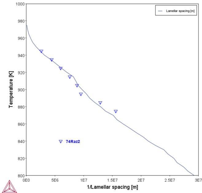
Figure 41: Lamellar spacing as a function of temperature.
