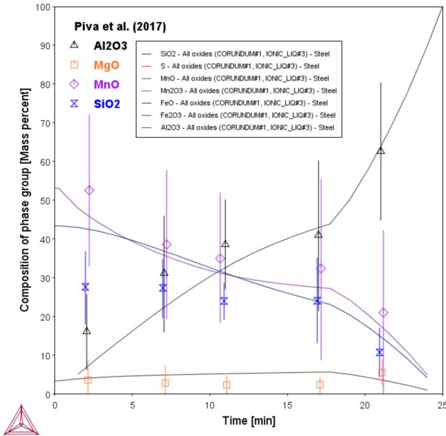
Figure 57: Calculated composition of non-metallic inclusions in function of processing time compared to experimental data [2017Piv].
