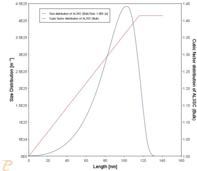
Figure 100: Particle size distribution (PSD) and cubic factor.
