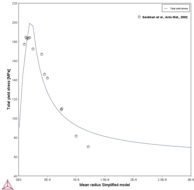
Figure 28: Strength vs Radius - Seidman compared to experimental data from [2002Sei].
