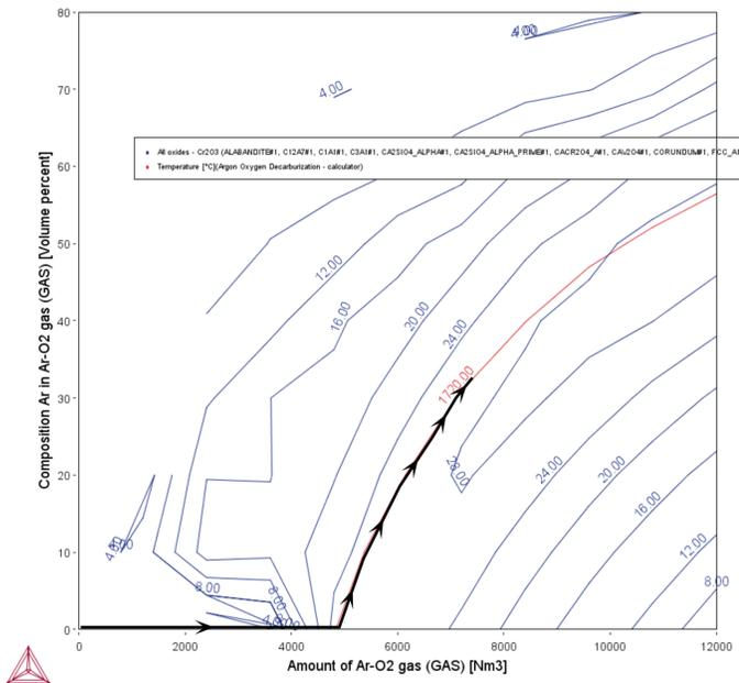
Figure 52: In the Cr Content in Slag plot, the Cr<sub>2</sub>O<sub>3</sub>-content in the slag reaches at the end of the process ca. 26 wt-%. This is typical for the AOD-process and requires an additional Cr-recovery step after the conversion to reduce the loss of chromium. The black line in the plot indicates a possible process control path that finally leads to suitable alloy composition close to a X5CrNi 18-10 stainless steel.
