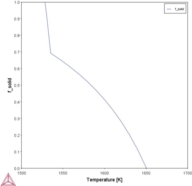
Figure 8: The result of the f\_solid function.
