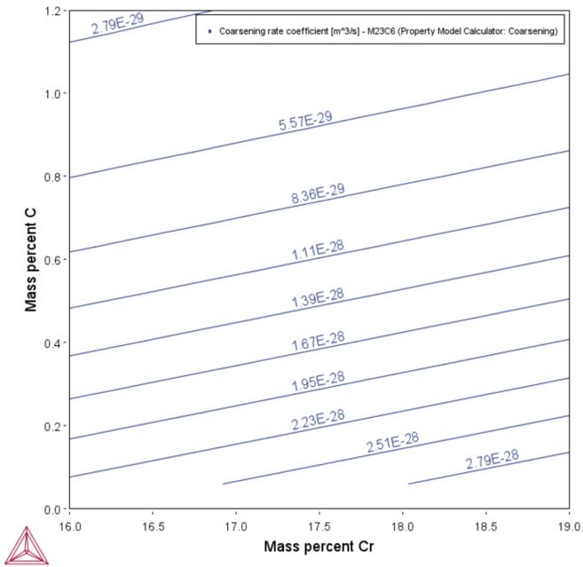
Figure 22: Coarsening rate coefficient (contour plot).
