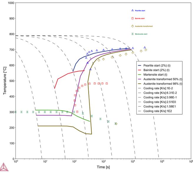
Figure 47: The CCT diagram for an Fe-C-Mn-Si-Cr-V alloy comparing the calculation with experimental data from [1958Wev].
