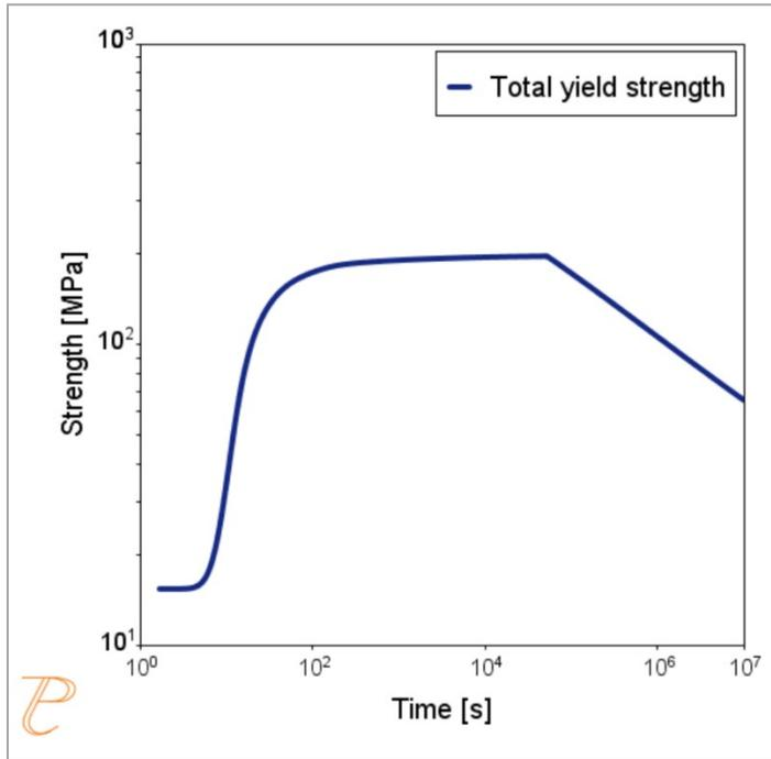
*This plot shows the yield strength of the AL3SC precipitate as a function of time.*
