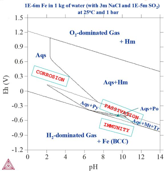
Figure 3: 1E-6 m Fe actively reacted with 1 kg of water, 3m NaCl and 1E-5 m SO<sub>2</sub> at 25° C and 1 bar. Introducing SO<sub>2</sub> into the system leads to the formation of various metal-sulphides (Py-pyrite, Popyrrhotite, Tr-troilite). In addition, the passivation region becomes larger.
