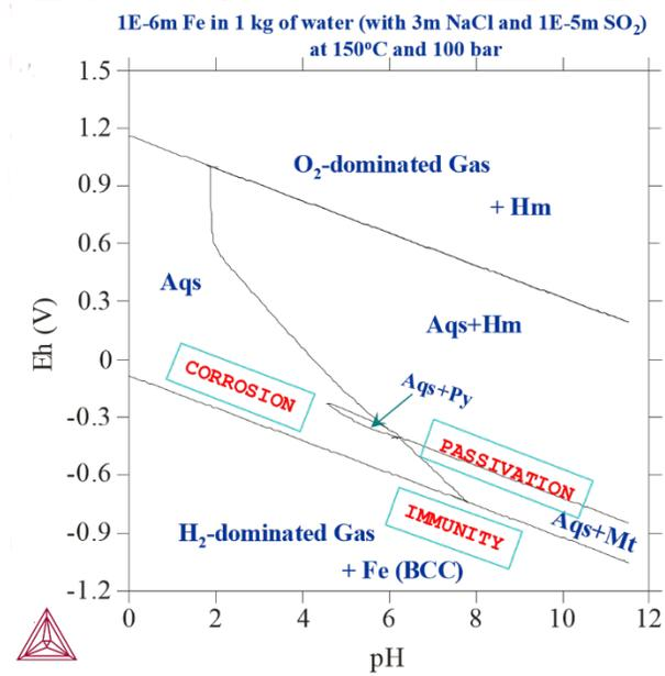
Figure 4: 1E-6 m Fe actively reacted with 1 kg of water, 3m NaCl and 1E-5 m SO<sub>2</sub> at 150° C and 100 bar. Here, changing the temperature and pressure affects the stability fields of various Fe-oxides/sulphides.
