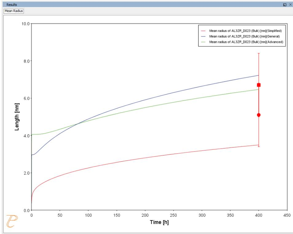
Result comparing the mean radius of the spheres for each AL3ZR\_D023 precipitate phase calculated for each type of growth rate model.
