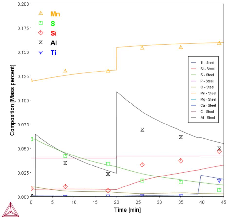
Evolution of the steel chemistry in function of time during ladle furnace treatment. Most of the experimentally measured datapoints are very well reproduced by this very simple model set-up demonstrating that the underlying processes are well captured. This plot is not included with the example but you can try to reproduce it yourself or go to our website to see the detailed example available there.
