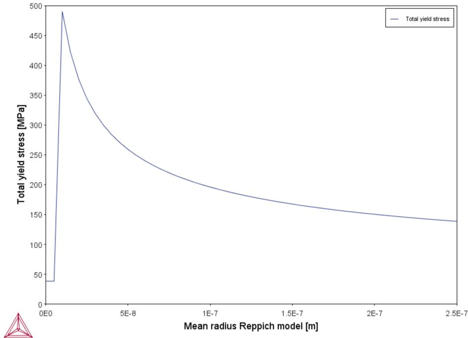
Figure 9: Reppich model yield strength vs mean precipitate radius for Ni-10Cr-10Al.
