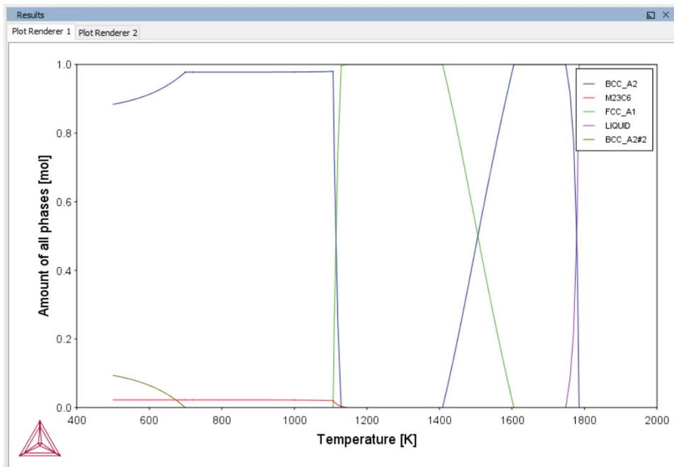
The Equilibrium Calculator and a One axis calculation is used to determine how the phases change with temperature.
