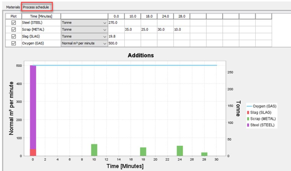
The Process schedule tab for a Process Metallurgy Calculator where you enter your steelmaking recipe.
