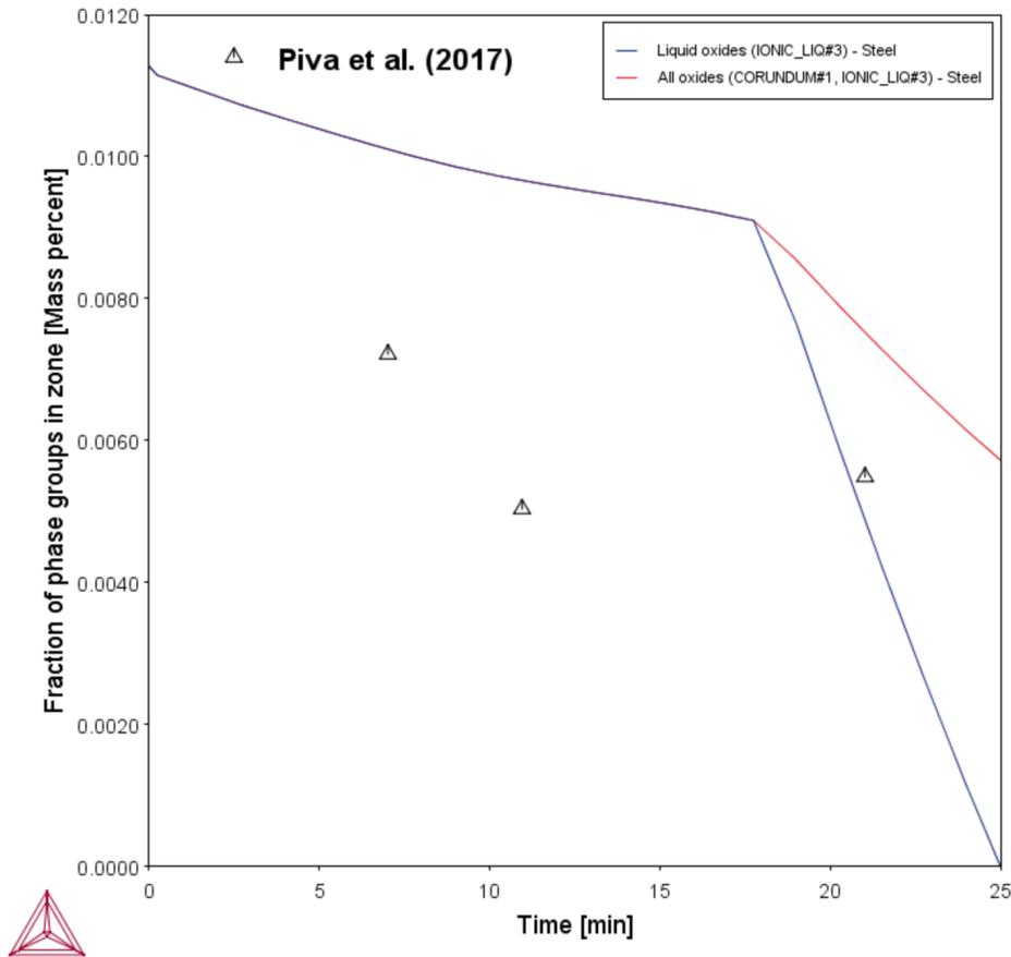
Amount of inclusions in the liquid steel in function of processing time. The total amount of inclusions (red line) and liquid oxide inclusions (blue line) are plotted. Up to about 20 min all inclusions are liquid oxide type, then they are replaced by solid corundum ( $Al_2O_3$ ) inclusions. Experimental data from Piva et al. [2017].
