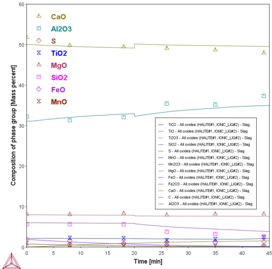
Evolution of the slag chemistry in function of time during ladle furnace treatment.
