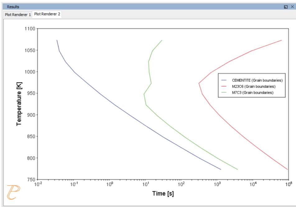
The Precipitation Calculator is used to do a TTT (Time-Temperature-Transformation) diagram calculation of the three phases (cementite, M23C6 and M7C3) at the grain boundaries.
