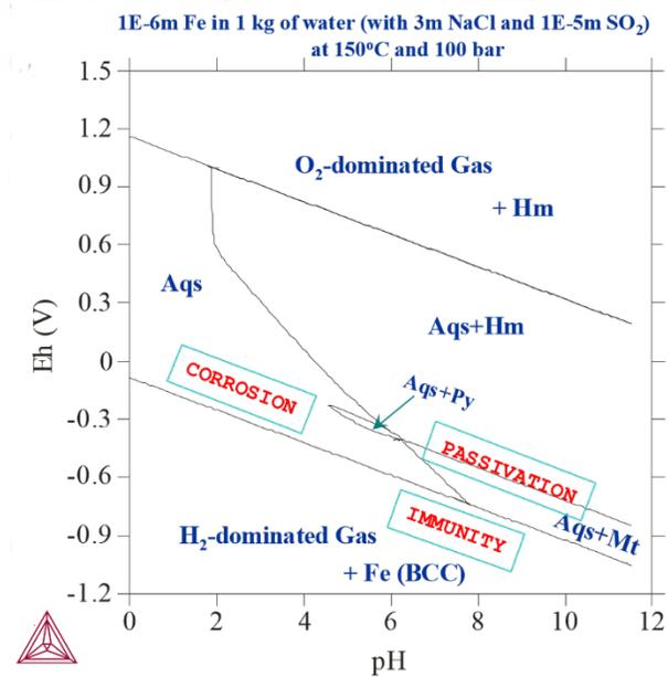
Figure 16: 1E-6 m Fe actively reacted with 1 kg of water, 3m NaCl and 1E-5 m SO<sub>2</sub> at 150° C and 100 bar. Here, changing the temperature and pressure affects the stability fields of various Fe-oxides/sulphides.
