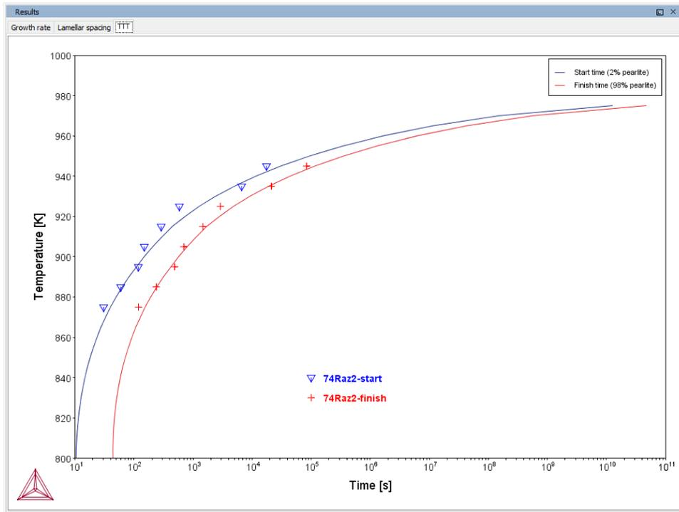
The TTT (time-temperature-transformation) diagram showing times of start (2% transformation) and finish (98% transformation) as functions of isothermal heat treating temperature in an Fe-0.69C-1.80Mn alloy (mass %).
