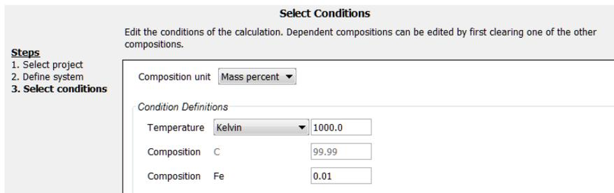
For a **One axis equilibrium** or **Phase diagram**, specify the **Axis Definitions** of the stepping or mapping operation. Choose minimum and maximum values for the variable(s) (select **Linear – min no. of steps**, **Linear – max step size** or **Logarithmic –scale factors**) and whether it is **Normal** or **Separate phases**. For a **Scheil solidification simulation**, and where applicable, select **Fast diffuser** to account for back diffusion of any fast-diffusing elements.
