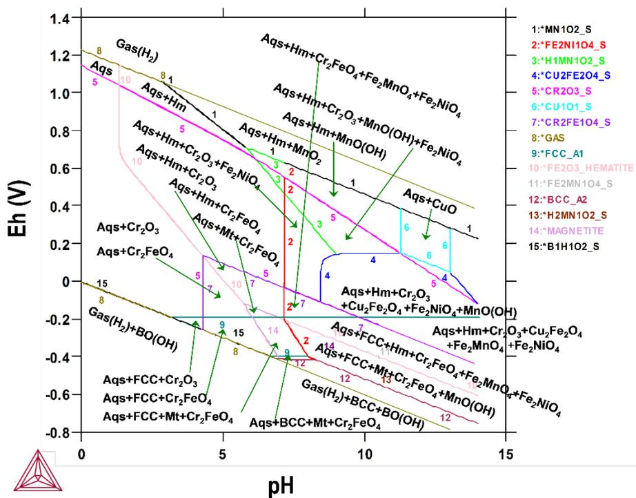
The next example is a Pourbaix diagram calculated for the heterogeneous interaction systems between 0.1 mole of AISI4340 stainless steel (Fe-0.80Cr-1.85Ni-0.70Mn-0.25Mo-0.25Si-0.40C [wt%]) and 1 kg of seawater (with the equivalent of 0.6054 m NaCl), at 25° C and 1 bar. This application is particularly useful for failure analysis of petroleum exploitation industry.
