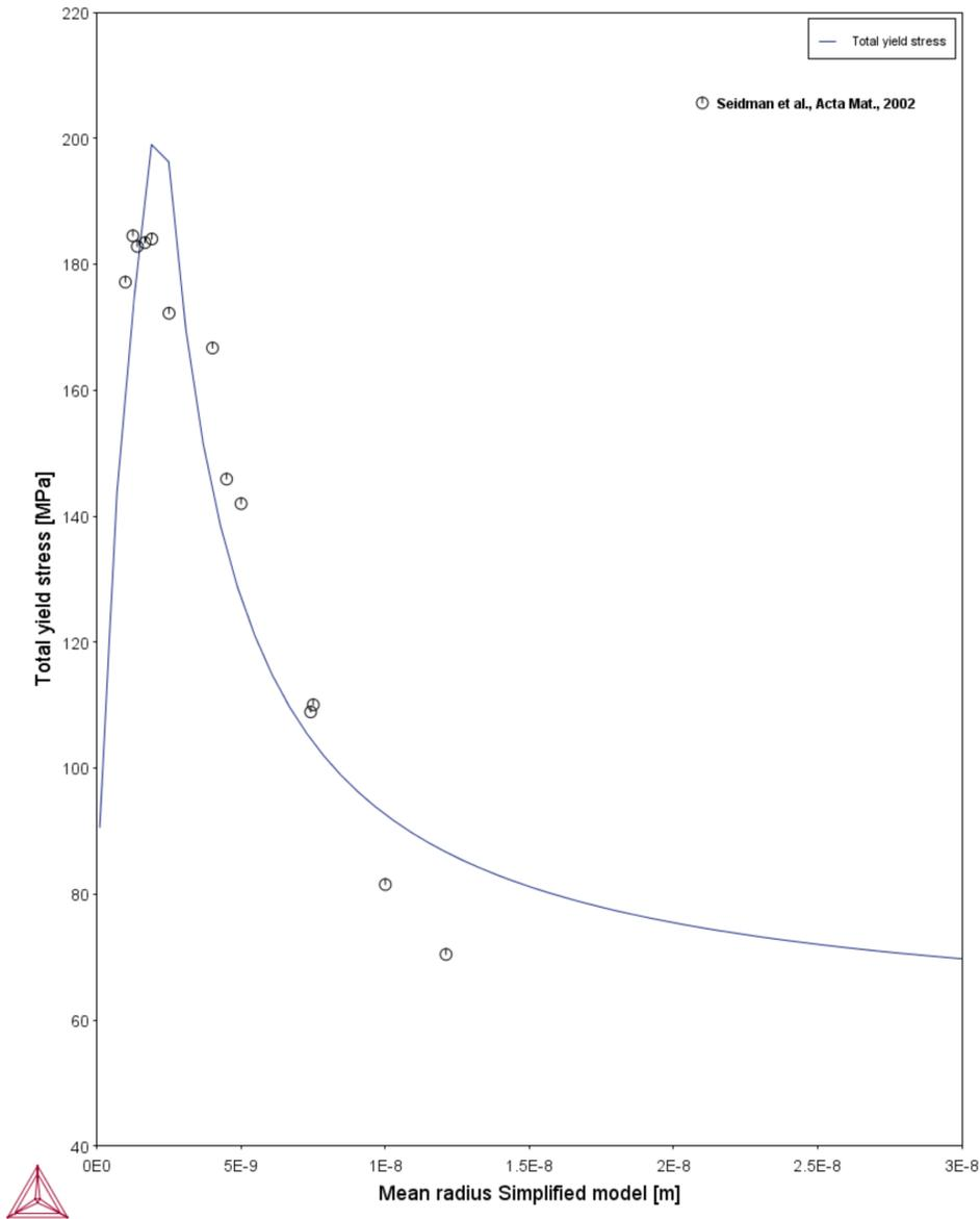
Figure 6: Yield strength Property Model plot example using the 'Simplified model' as described in the text.
