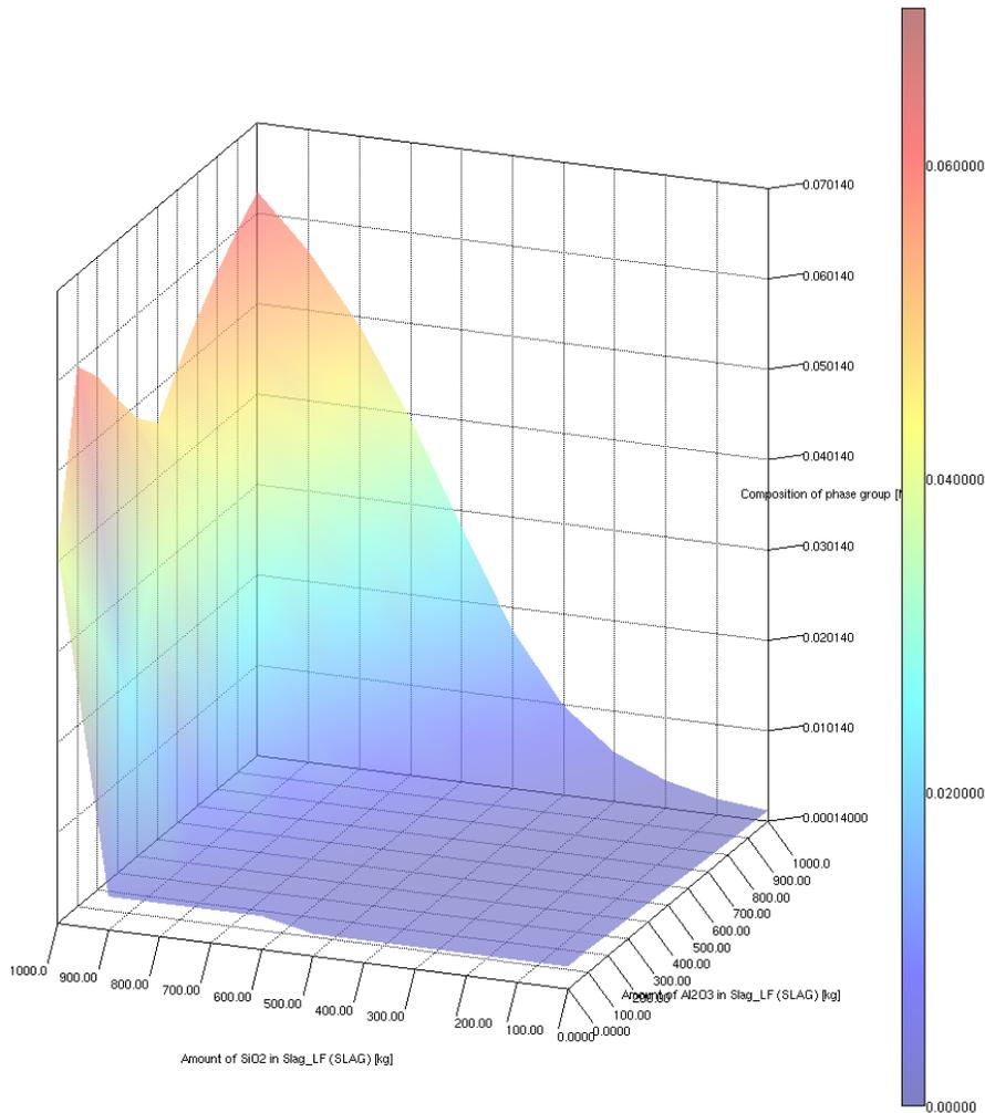
Refer to the *Sulfur in liquid steel* 3D plot included with the example. The red colors in the upper right-hand corner at high SiO<sub>2</sub> and Al<sub>2</sub>O<sub>3</sub> content show that the steel contains high amounts of sulfur.
