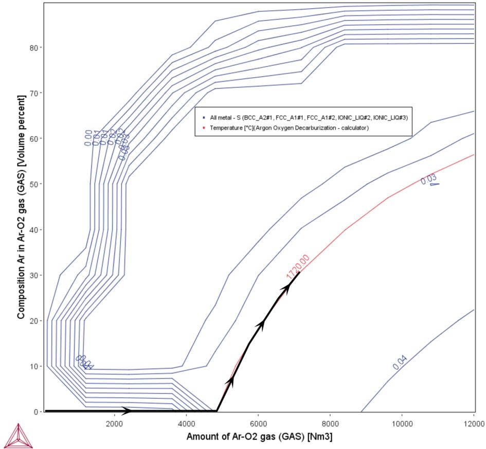
In the S Content in Steel plot, the sulphur content in the steel melt is slightly reduced during the process from 0.056% in the initial steel scrap to finally ca. 0.035%. The black line in the plot indicates a possible process control path that finally leads to suitable alloy composition close to a X5CrNi 18-10 stainless steel.
