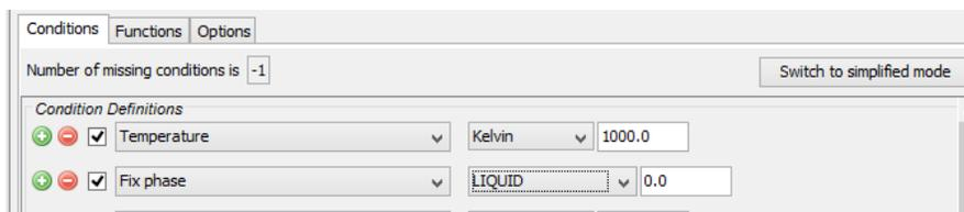
Above the *Condition Definitions*, the **Number of missing conditions is** field is probably **-1**. This means that you must remove one condition.
