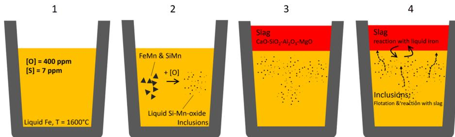
*Diagram of the experiment performed by Piva et al. [2017]. The sequence as described in the text is: (1) liquid Fe with dissolved oxygen; (2) FeMn and SiMn added to deoxidize Fe; (3) top slag added after 360s; and (4) gradual reaction between steel, slag and inclusions.*
