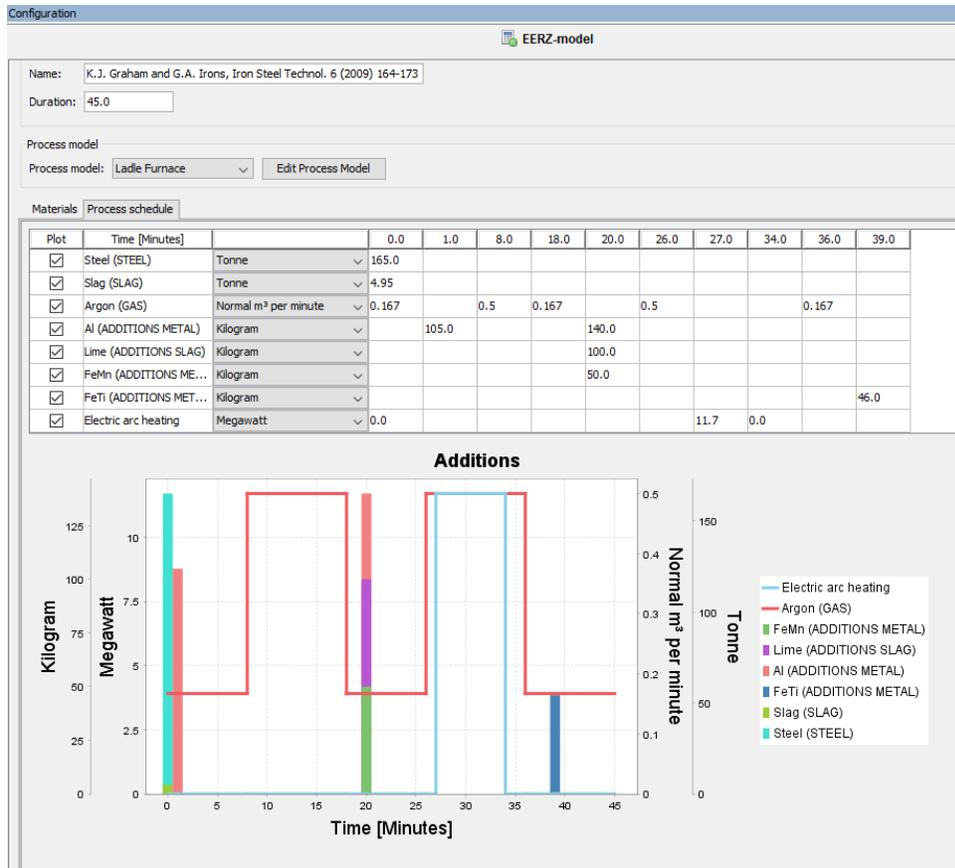
The Process schedule set up for this example. If you have the project open in Thermo-Calc, click the Process schedule tab to view this. You can then click the check boxes in the Plot column to include or exclude materials to better visualize the process schedule on this tab. This is based on the LF steel refining process schedule as published by Graham and Irons [2009, Graham].
