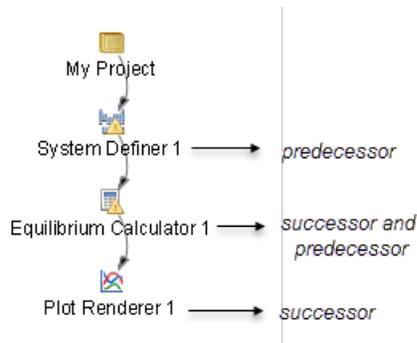
For example, to calculate and display a phase diagram, create a branch with three linked activities: A **System Definer** activity linked to an **Equilibrium Calculator** activity, which in turn is connected to a **Plot Renderer** activity.
