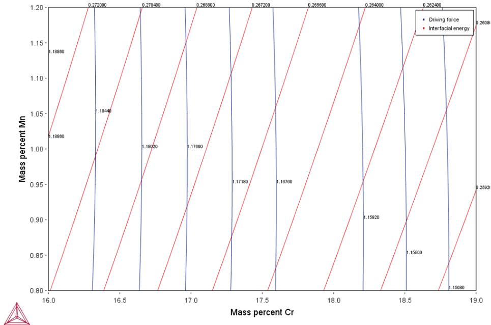
A contour plot showing both the driving force and interfacial energy calculation results comparing Mass percent Cr to Mass percent Mn.
