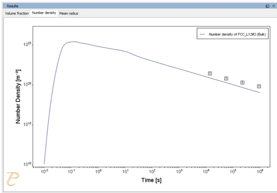
The results of an isothermal calculation to plot the number density of the cementite phase.
