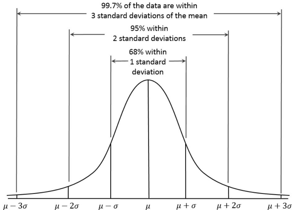
As long as the number of events (the sample size) is very large, then the Gaussian distribution function can be used to describe physical events. A Gaussian distribution is assumed to describe how each quantity varies in an uncertainty calculation, as shown next.
