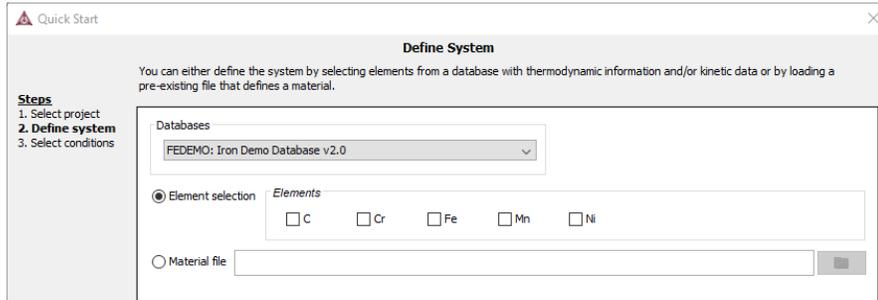
4. Click to select **Elements** check boxes to include as system components. To add elements from an existing material file, click the **Material file** button to enter the file path to a material file or click the **Select Material File** button (to the right of the field) to navigate to a file on the computer.
