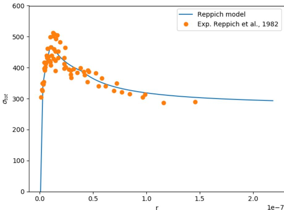
Figure 8: Reppich model plotted with results and experimental data for PE16 [1982b, Reppich], all data is normalized with the square root of the volume fraction of precipitate.
