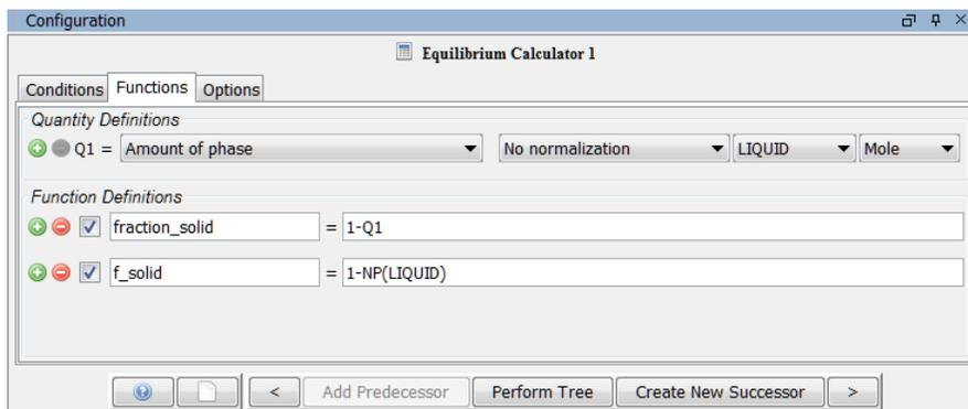
4. Under **Function Definitions**, click the add button to add a new function. In the left field edit the default name of each function and enter the function itself in the right field after the equal sign. In this example, the quantity defined as Q1 is renamed to **fraction\_solid**, which gives as its output the fraction of solid phase (**1-Q1**).
