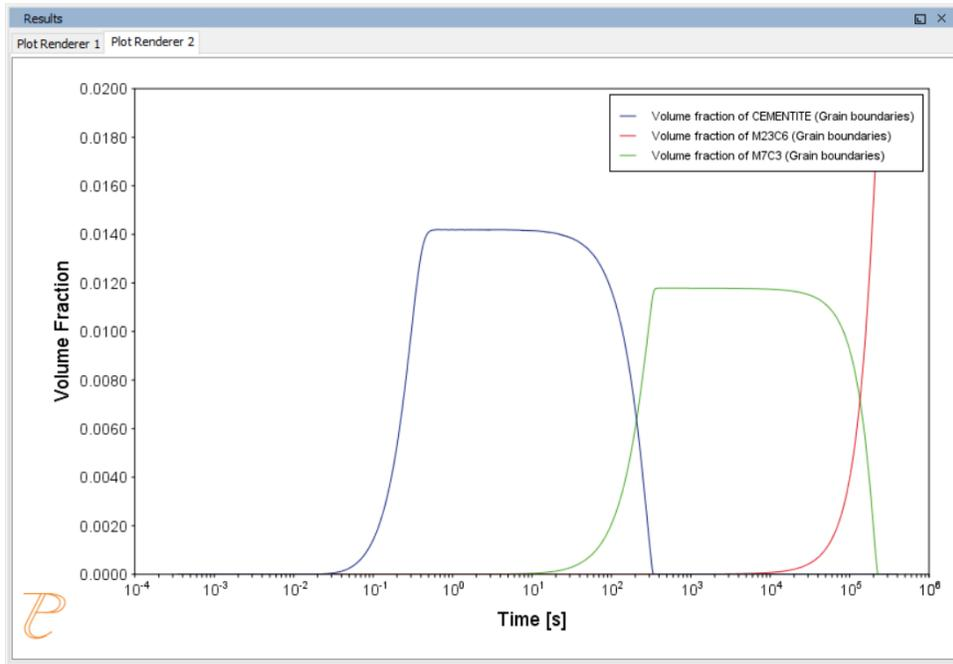
The Precipitation Calculator is used to do an isothermal calculation of the three phases (cementite, M23C6 and M7C3) where cementite and M7C3 are metastable phases.
