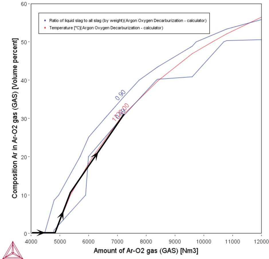
In the Liquid Slag Fraction plot, you can see that towards the end of the process the slag is calculated to be mostly liquid. The black line in the plot indicates a possible process control path that finally leads to suitable alloy composition close to a X5CrNi 18-10 stainless steel.
