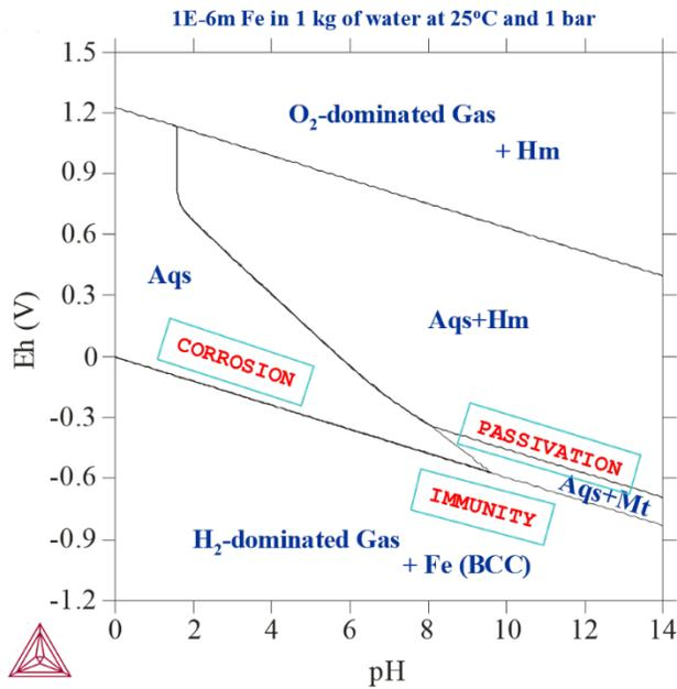
Figure 14: 1E-6 m Fe actively reacted with 1 kg of pure water at 25° C and 1 bar. Note that the active metal corrosion region gets enlarged as the initial Fe amount decreases from 1E-3m to 1E-6m.
