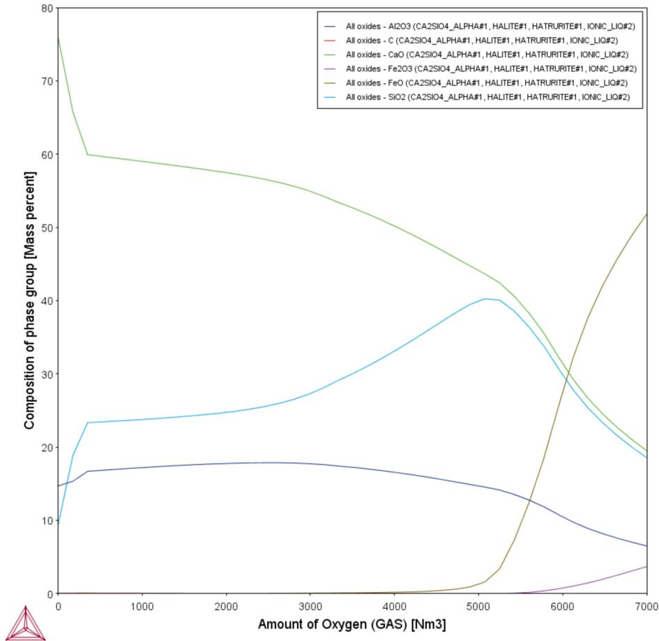
This plot shows how the liquid slag composition changes as a function of the amount of oxygen added to the BOF.
