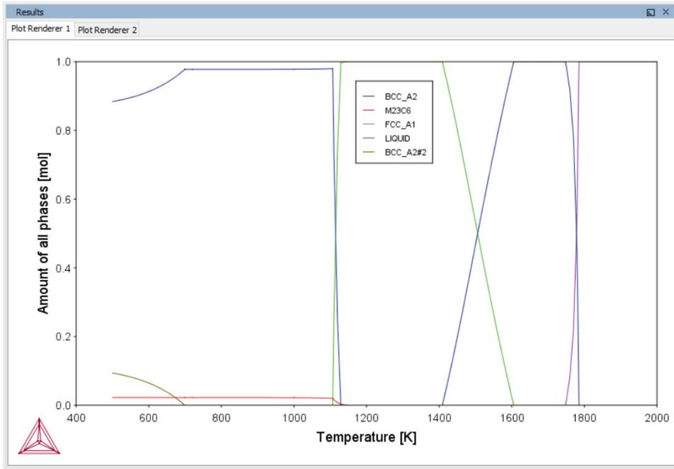
The Equilibrium Calculator is used to show how the phases change with temperature.
