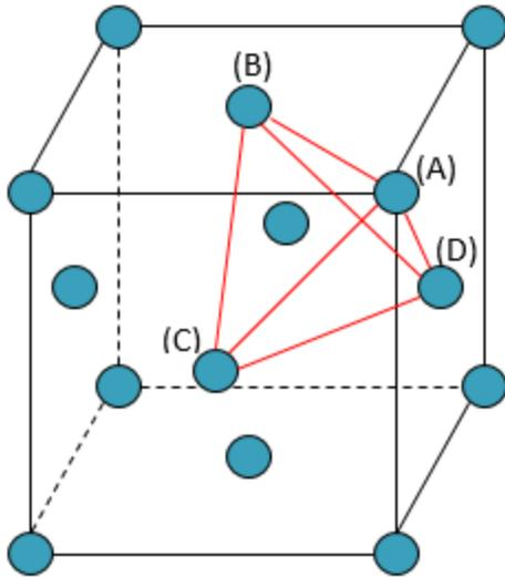
A *Normal 4-Sublattice Model* requires that all the  $G$  parameters for each of the end-members with the same elements but distributed on different sites be given separately. However, as these corners are identical lattice points, the phase-type option  $F$  means that the  $G$  parameters need be given only once. The possible permutations are handled automatically.
