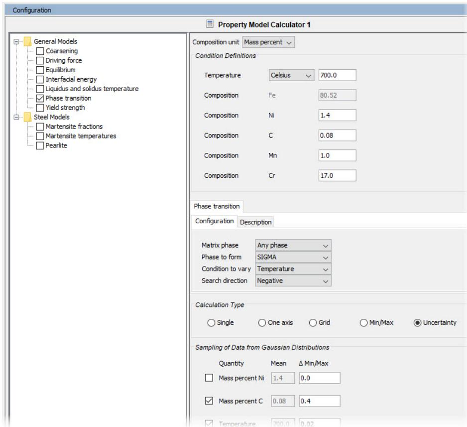
An example of the Configuration window settings when using a Phase Transition Model and an Uncertainty calculation type.
