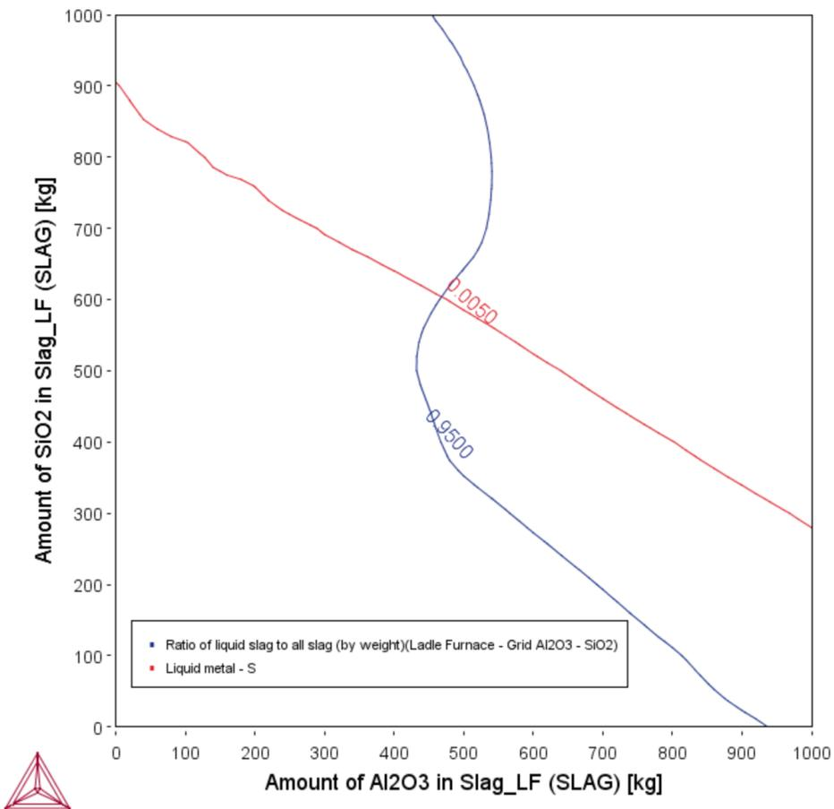
The optimal slag has a composition delimited by these two contour lines, so below the contour line for sulfur content in the liquid steel and above the contour line for fraction of liquid slag will be both fully liquid and effectively desulfurizes the steel.
