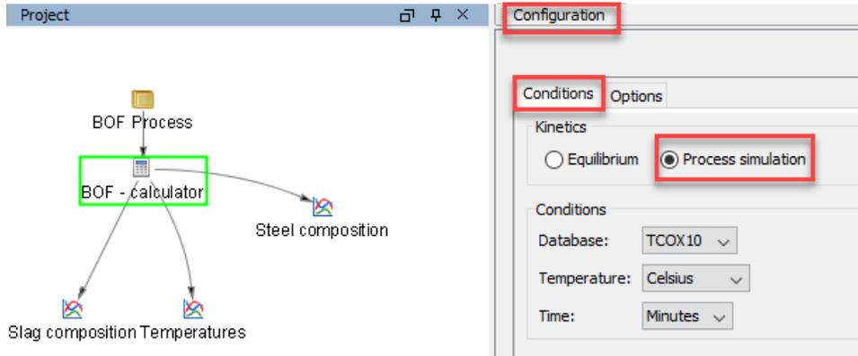
The Process Metallurgy Calculator for this example is renamed *BOF - Calculator* in the Project window. To the right is the Configuration window where you choose to define a Process simulation.
