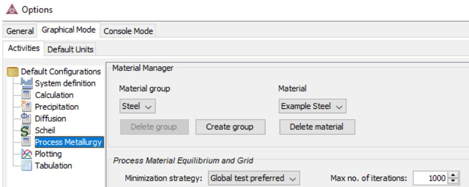
For frequently used materials, save the material composition for each group—*Steel* (or any user-defined metal), *Slag* or *Gas*—from the *Process Metallurgy Calculator*. Use the *Material Manager* to create and delete groups or delete a previously saved material.
