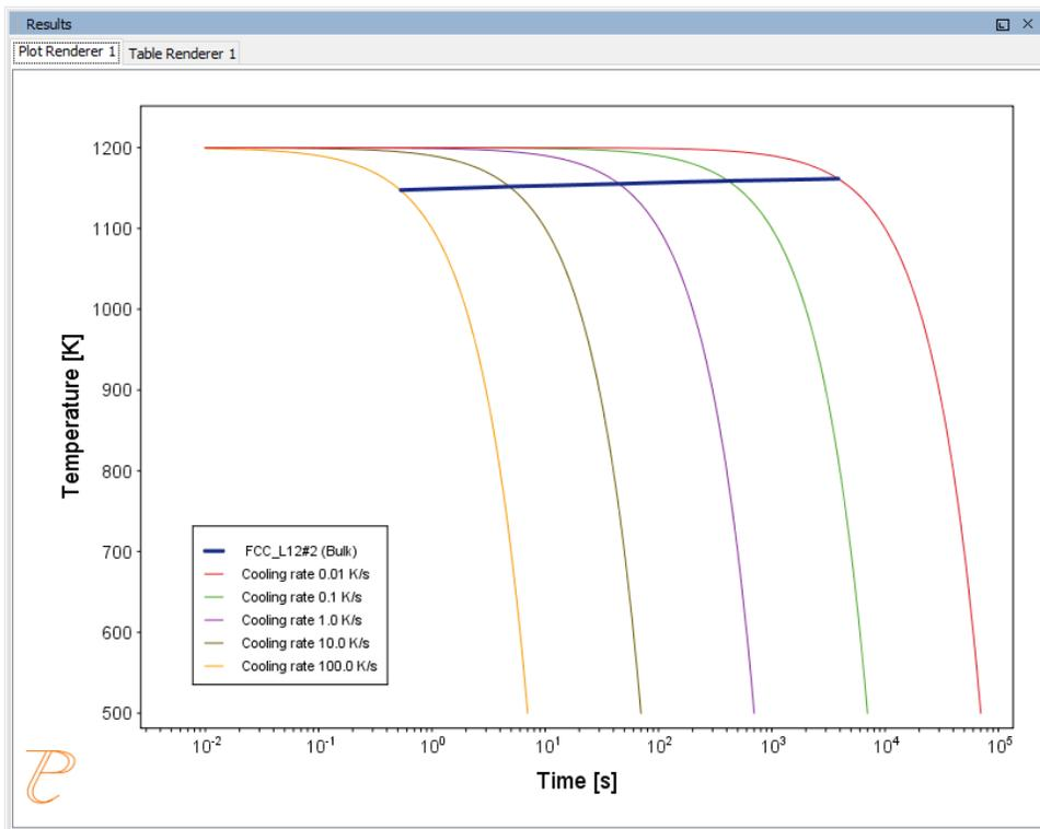
In this plot, the blue line shows the time it takes for  $\gamma'$  to transform at each of the cooling rates according to the stop criteria, which we set as  $1e-4$  volume fraction. The cooling rates are represented by the multi-coloured curved lines.
