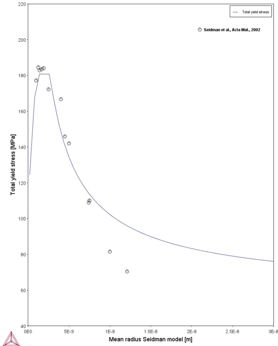
Figure 7: Yield Strength Property Model plot example using the 'Seidman model' as described in the text [2002, Seidman].
