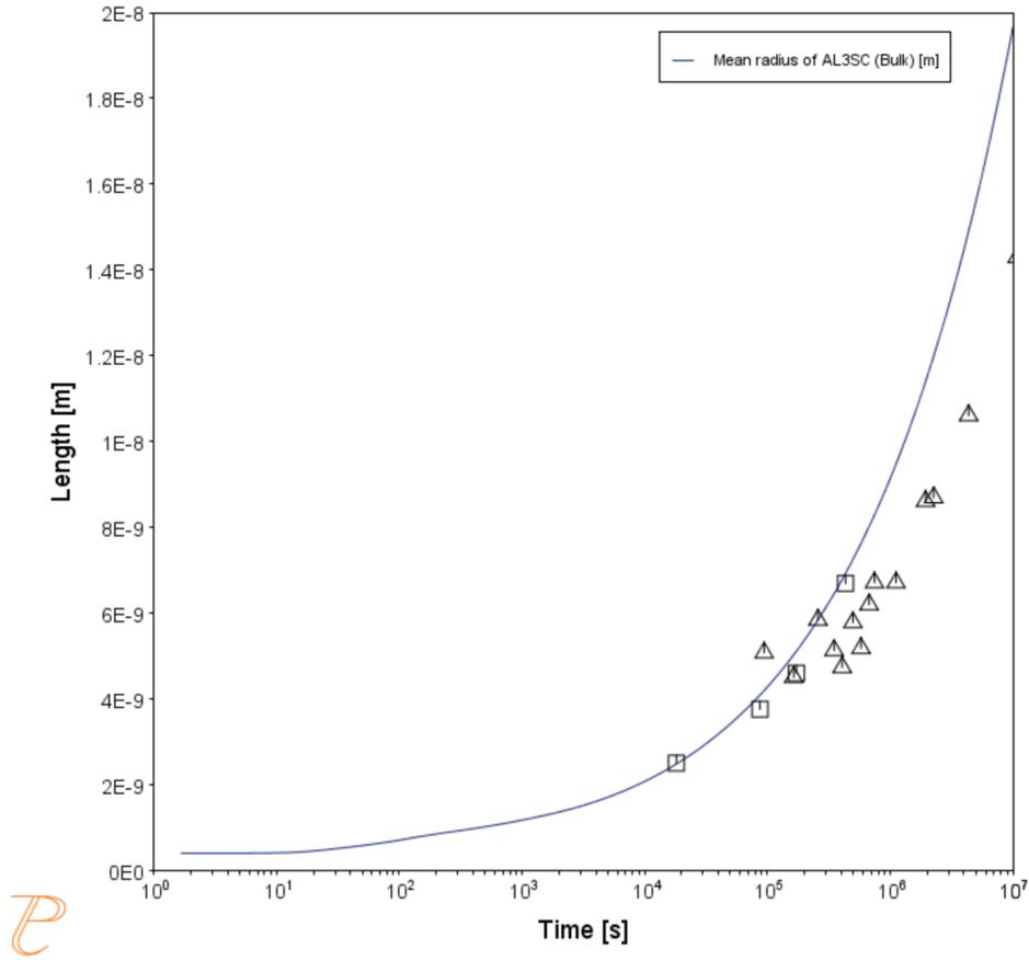
This plot shows the mean radius of the AL3SC precipitate as a function of time.
