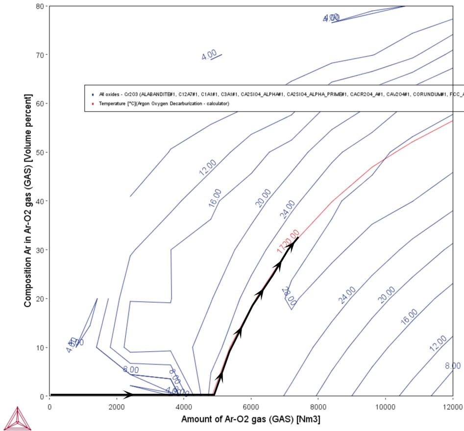
In the Cr Content in Slag plot, the Cr<sub>2</sub>O<sub>3</sub>-content in the slag reaches at the end of the process ca. 26 wt-%. This is typical for the AOD-process and requires an additional Cr-recovery step after the conversion to reduce the loss of chromium. The black line in the plot indicates a possible process control path that finally leads to suitable alloy composition close to a X5CrNi 18-10 stainless steel.
