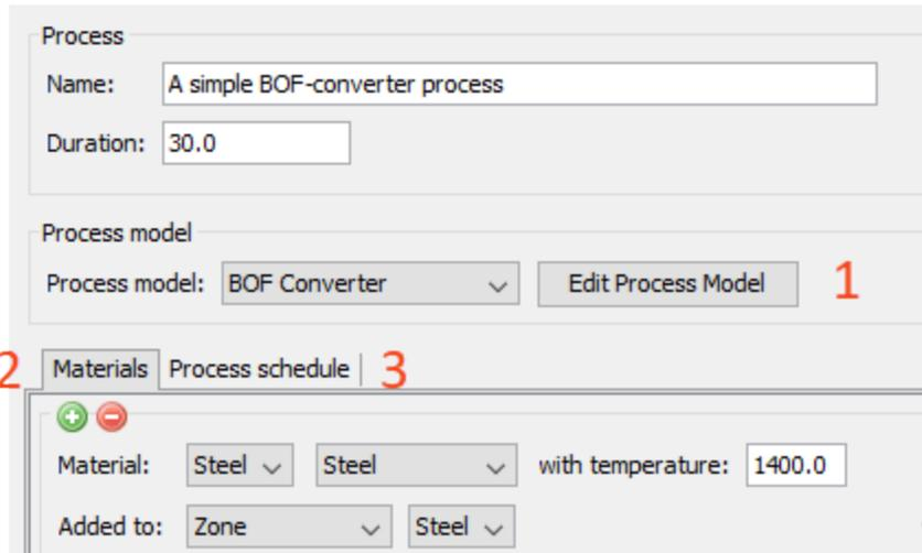
The settings you need to access are on the Process Metallurgy Calculator Configuration window. From here, you perform three steps to set up a kinetic simulation. (1) Edit the Process Model, (2) Define the Materials, and then (3) Define the Process Schedule.
