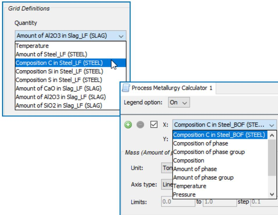
After defining and saving a material composition, the named material is available for selection in a variety of places such as when choosing quantities on the calculator and defining axis variables on the Plot Renderer.
