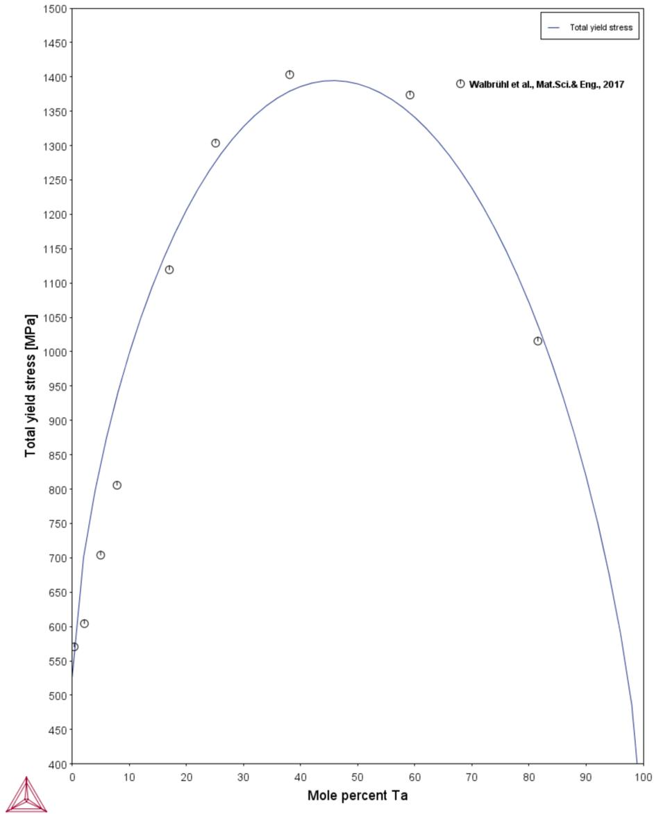
Figure 5: Yield strength vs Ta-content for the binary high entropy Mo-Ta alloy.
