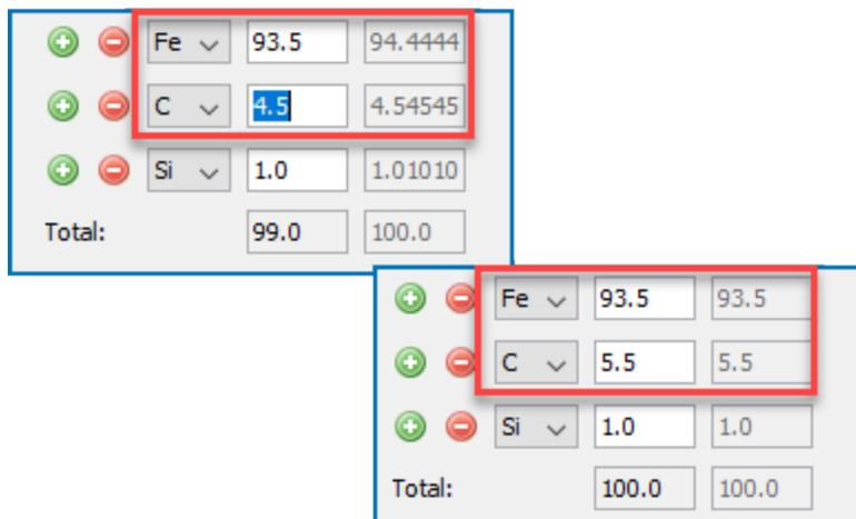
Sometimes its preferable to use input of amount of each component **Amount** by weight (**Tonne, Kilogram, Gram** or **Pound**), it can useful to choose **Absolute amount** as the **Input type**. In this case, the total amount of material automatically adjusts the total.
