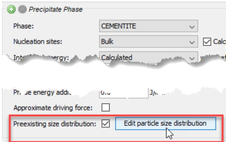
3. Click **Edit particle size distribution** to open the window as shown for example P\_10.
