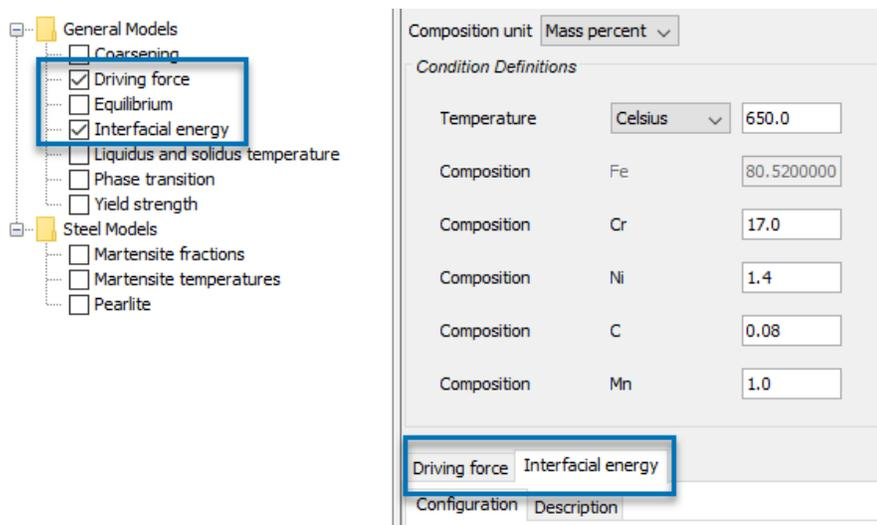
3. Enter the settings described in [Configuration Window Settings](#) and for each *Calculation Type* (Single, Grid, Min/Max, and Uncertainty).
