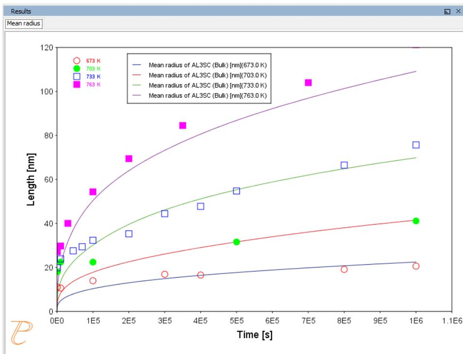
The results of an isothermal calculation to examine the mean radius of an Al-0.12Sc system.
