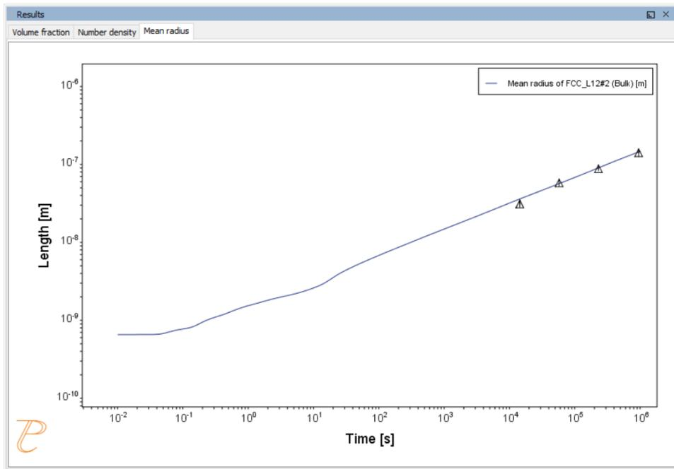
The results of an isothermal calculation to plot the mean radius of the cementite phase.
