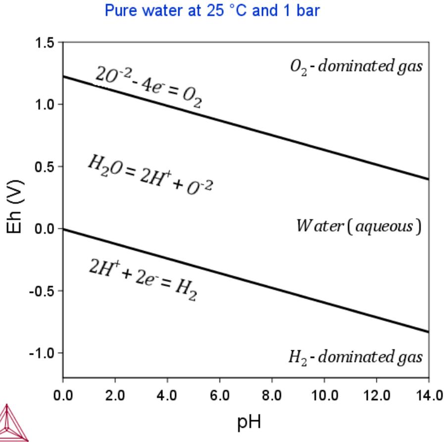
Figure 11: A pH-Eh diagram for pure water at 25 °C and 1 bar.
