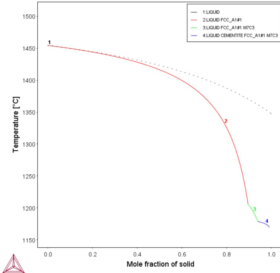
After the Scheil-Gulliver solidification simulation runs, the diagram Temperature versus Mole Fraction of Solid is plotted in the Console Results window.
