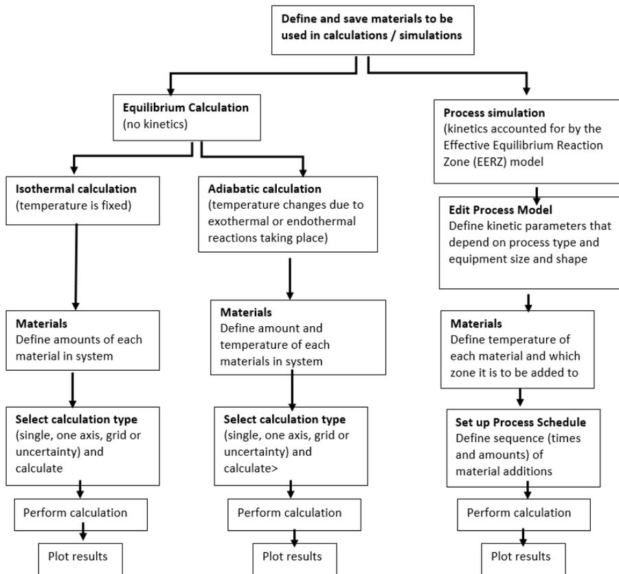
The three branches of simulations available for the Process Metallurgy Calculator (1) an isothermal equilibrium calculation (2) an adiabatic equilibrium calculation and (3) a process simulation.
