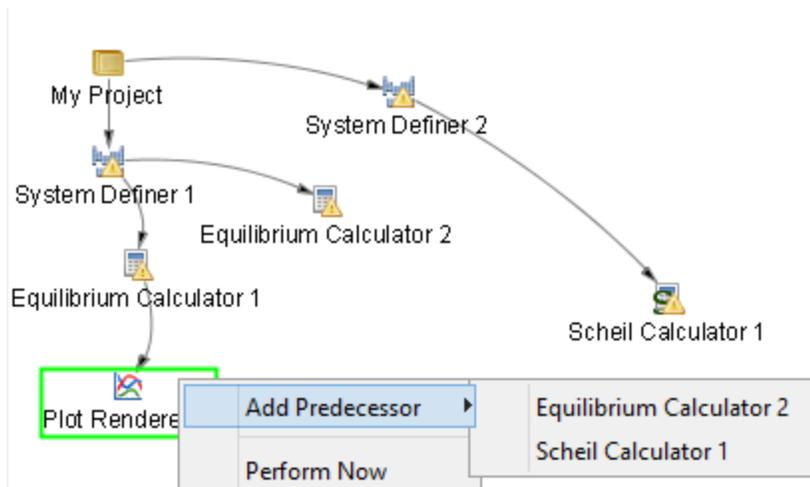
3. Select a predecessor. When added, the extra predecessor is linked to the Plot Renderer. On the Plot Renderer's Configuration window, the predecessors are shown as two tabs:
