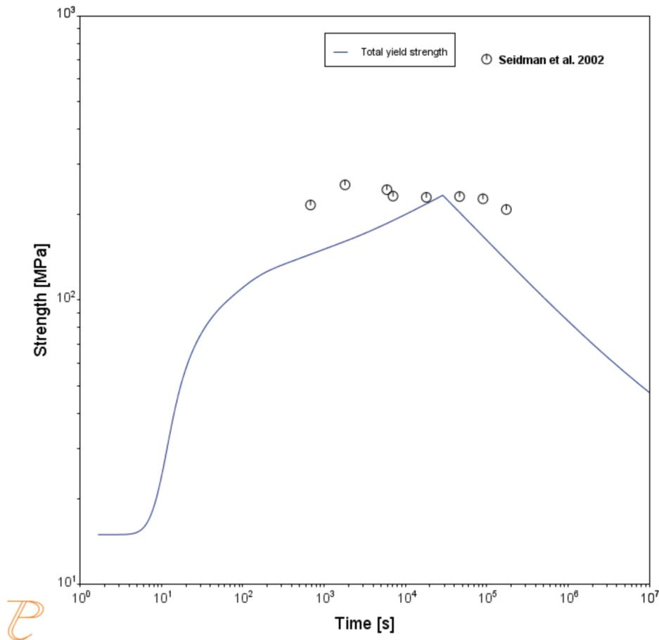
This plot shows the total yield strength of the AL3SC precipitate as a function of time compared to experimental data from Seidman et al. [2002, Seidman].
