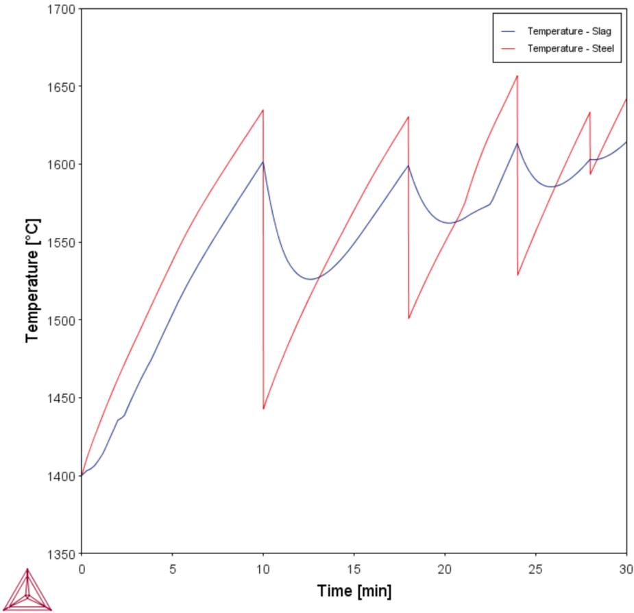
This plot shows the temperatures of the steel and slag bulk zones.
