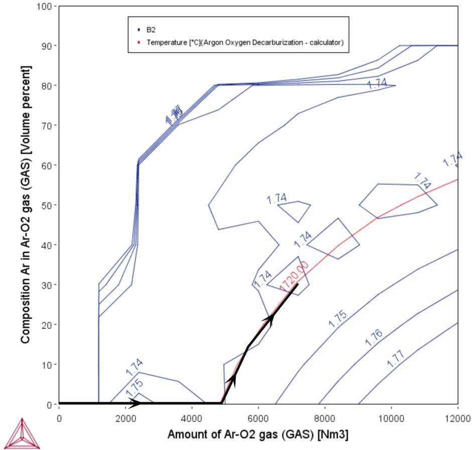
The Slag Basicity plot shows the basicity of the slag (which is a measure for the sulphur capacity of the slag). The process achieves a final basicity of 1.74 which is typical for an AOD-process. The black line in the plot indicates a possible process control path that finally leads to suitable alloy composition close to a X5CrNi 18-10 stainless steel.
