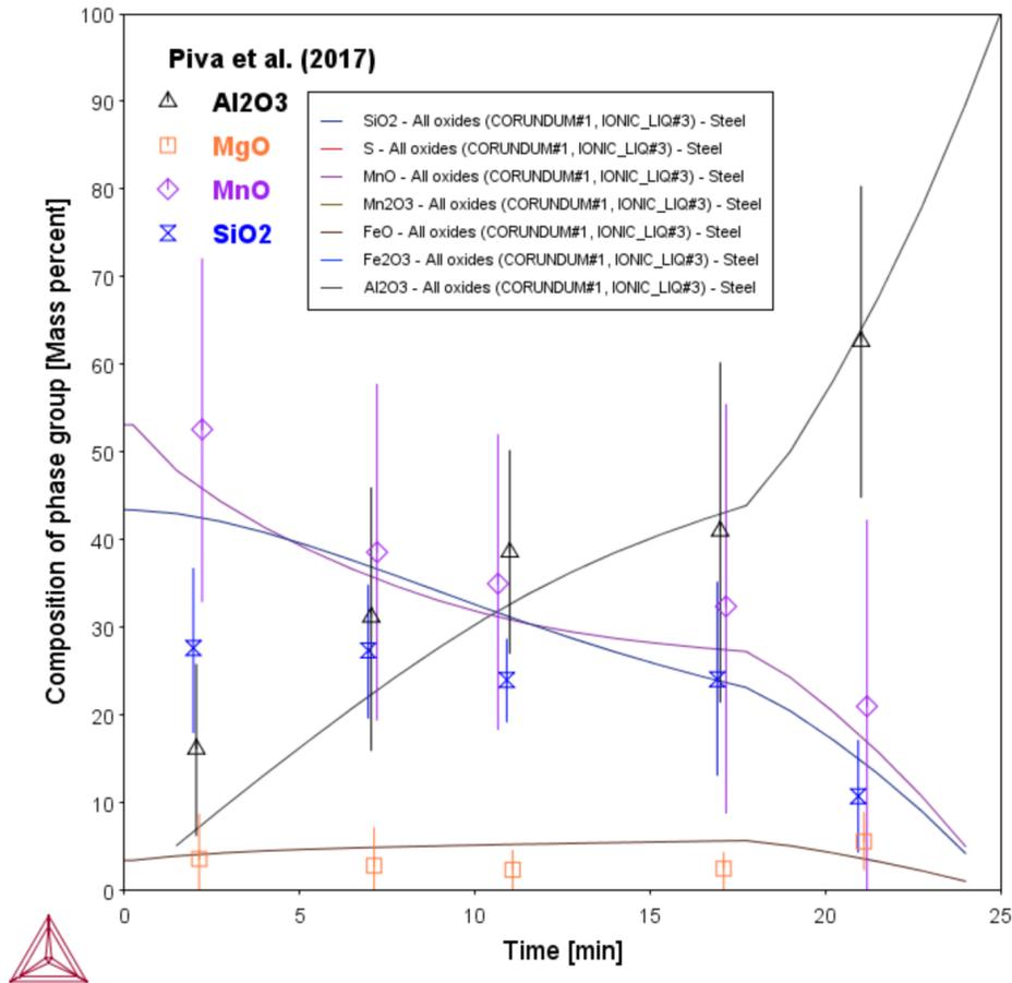
Calculated composition of non-metallic inclusions in function of processing time compared to experimental data [2017, Piva].
