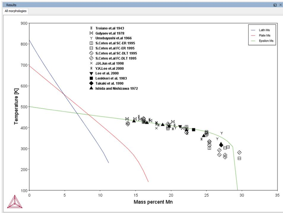
A diagram showing all the Ms temperatures of different types of martensite morphologies (lath, plate and epsilon (hcp) compared with experimental epsilon Ms values.
