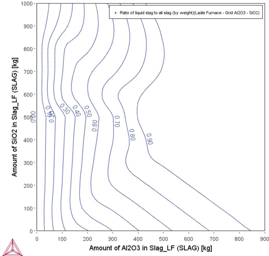
The plot shows that for low amounts of aluminium oxide ( $\text{Al}_2\text{O}_3$ ) and silicon dioxide ( $\text{SiO}_2$ ), almost no liquid slag is present. Process metallurgists refer to this as a *hard slag*.
