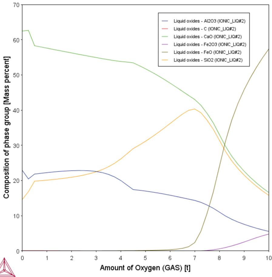
This plot shows how the liquid slag composition changes as a function of the amount of oxygen added to the BOF.
