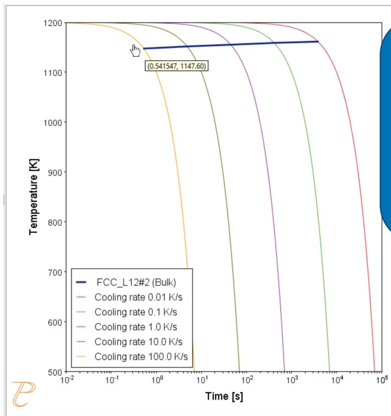
In this plot, the blue, horizontal line shows the time it takes for gamma prime to transform at each of the cooling rates according to the stop criteria, which we set as 1e-4 volume fraction.
