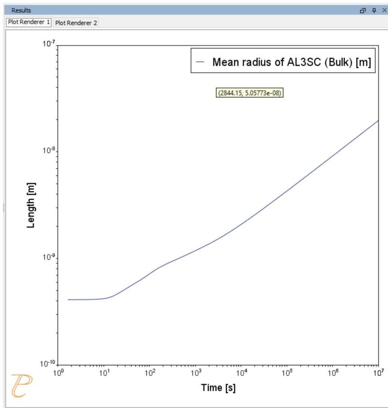
*This plot shows the Mean radius of the AL3SC precipitate as a function of time.*
