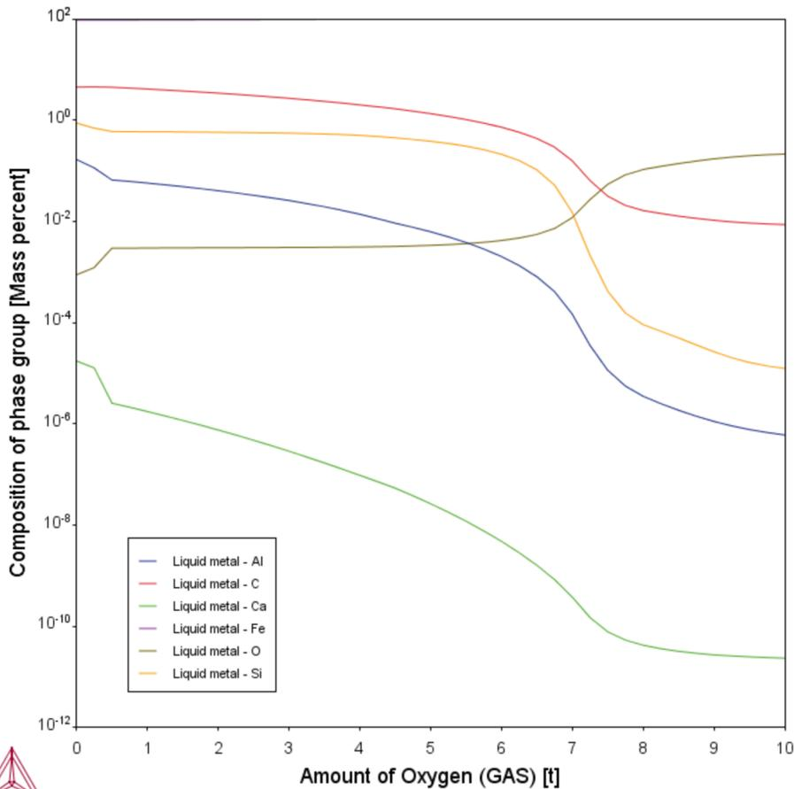
Now you can see the removal of the elements from the liquid steel in the following order: first calcium, then aluminium, then silicon and finally carbon (Ca, Al, Si and C) according to their position on the Ellingham diagram.
