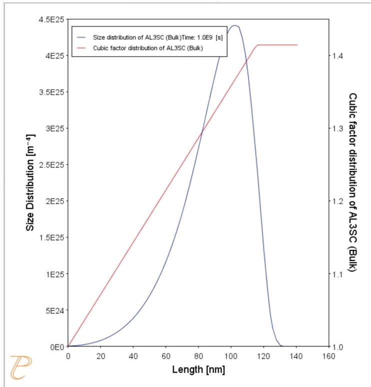
In this plot, the blue curve shows the particle size distribution and the red line shows the cubic factor distribution.
