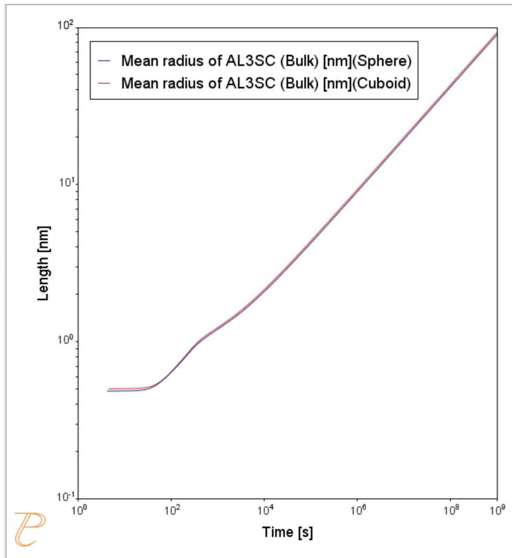
In this plot, the blue line represents the sphere calculation and the red line represents the cuboid calculation. You can see that, in this instance, they are almost identical.
