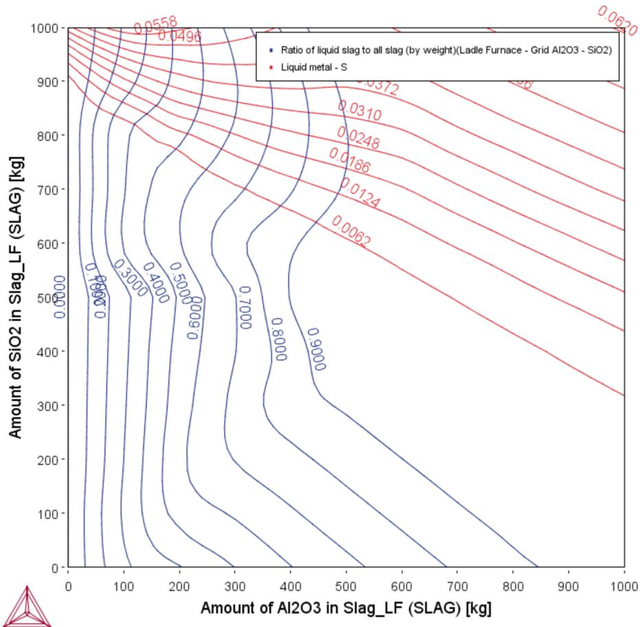
To map this optimal composition field one more plot can be generated by superimposing contour plots of sulfur content in the liquid steel and fraction of liquid slag.
