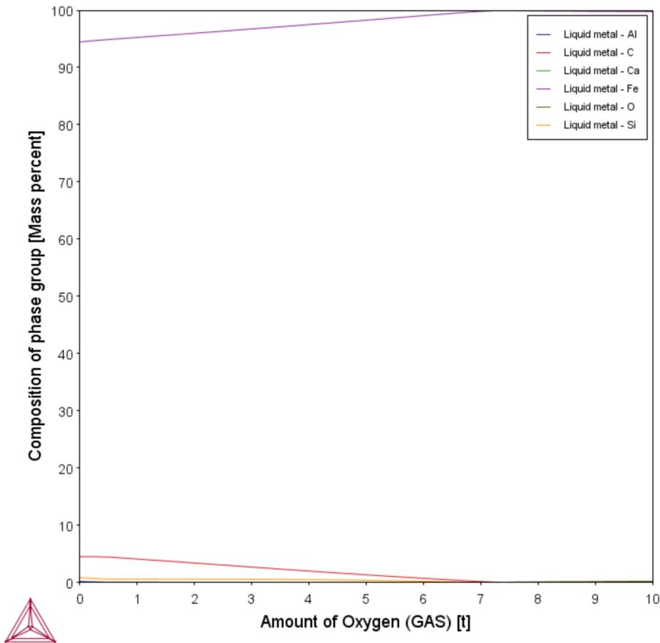
In the plot (that uses a linear axis) the reduction of the carbon content can be clearly seen. This reduction of the carbon content is what is termed “steelmaking”. The hot metal coming from the blast furnace has a very high carbon content of typically 4.5 wt%. If it is left to solidify without lowering the carbon content, it will be extremely brittle and be unfit for rolling or forging.
