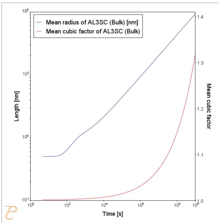
In this plot, the blue line represents the evolution of the average radius of the cubic particles as a function of time. The red line shows the average cubic factor as a function of time.
