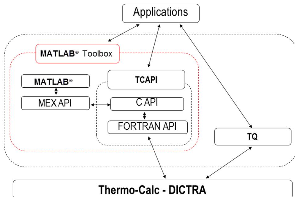
To be able to call MATLAB from programs written in C or FORTRAN there are MEX-files (MATLAB Executable) included with the MATLAB software. These MEX-files were utilised when interfacing MATLAB with Thermo-Calc.
