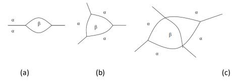
Figure 1: Non-spherical particles ( $\beta$ ) that precipitate at grain boundaries of matrix phase( $\alpha$ ) (a) grain boundary (two-grain junction) (b) grain edge (three-grain junction) (c) grain corners (four-grain junction). Images taken from Zang (2004)<sup>2</sup>.
