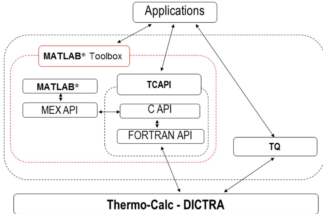
**Figure 1. Interfacing with the Thermo-Calc Engine.**
