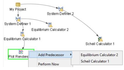
When selected, the extra predecessor becomes linked to the Plot Renderer in the "Project" window. On the Plot Renderer's "Configuration" window, the different predecessors are shown as two different tabs:
