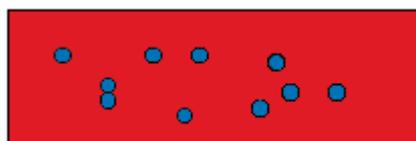
There are two ways in which you can simulate diffusion in a system that contains a dispersed phase, but it is strongly recommended that you use the so-called homogenization model. The homogenization model allows you to take into account diffusion in all phases for which you have kinetic data; the homogenization model treat all phases in the same way regardless of which phase was entered as type matrix and which phases were entered as type spheroid.
