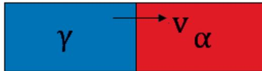
Normally, simulations in DICTRA are performed under the assumption that thermodynamic equilibrium holds locally at all phase interfaces. However, it is also possible to simulate a moving phase boundary problem while assuming that para-equilibrium conditions apply at the phase boundary.
