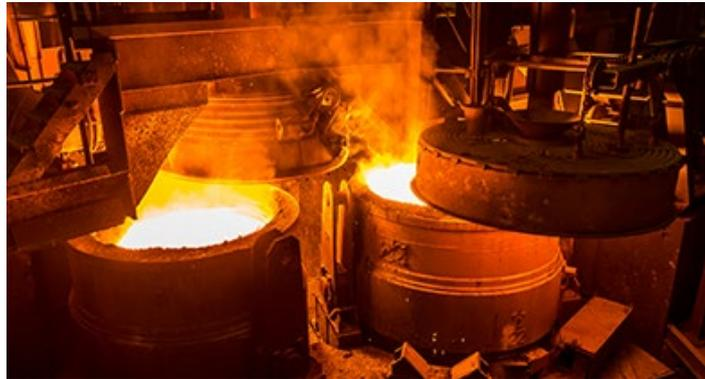
Figure 1. The principle of desulphurization is to transfer the sulphur dissolved in the liquid steel to a CaO-rich slag phase. This process is typically carried out in a ladle furnace (LF). Image of the ladle furnace at Swiss Steel ([www.swiss-steel.com](http://www.swiss-steel.com)).
